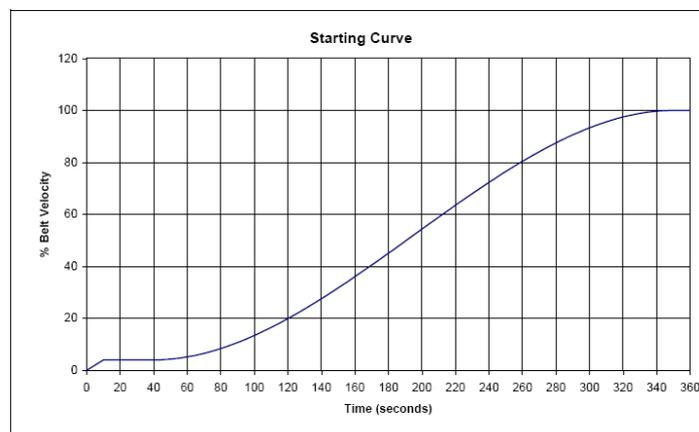
Figure 1. Typical Hermite S-curve for starting of long overland conveyors
