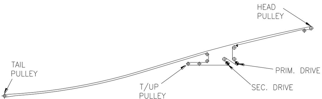
Figure 2. Layout of the head and drive end of the incline conveyor
