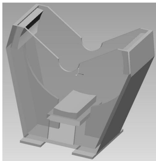
Figure 8. CAD model of catcher with transparent sides in order to view internal structure.
