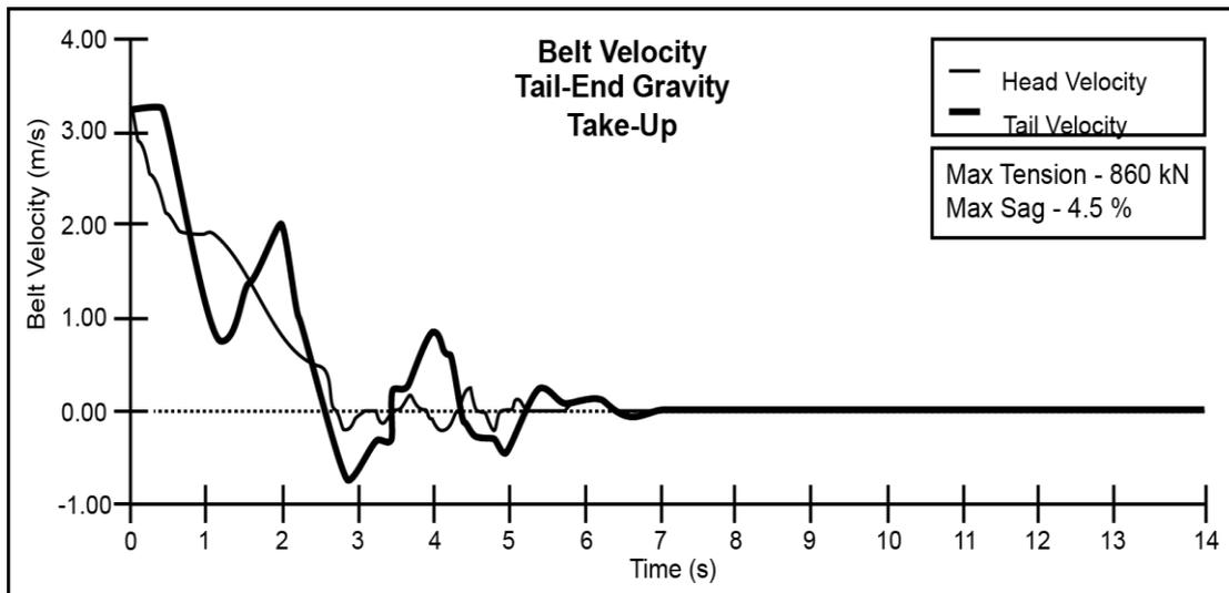
Figure 7. Belt speed with tail gravity take-up (emergency stop) [5]
