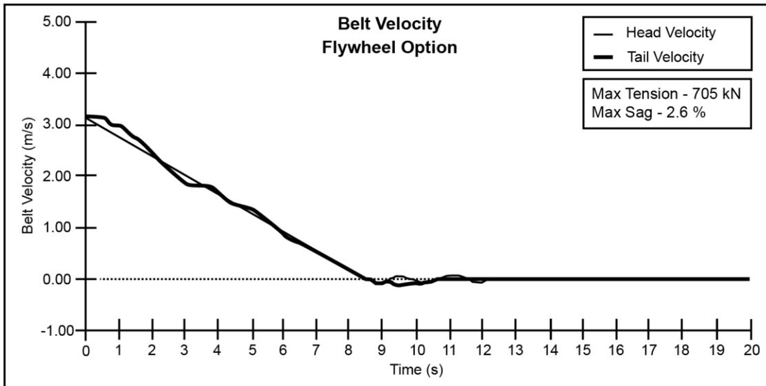
Figure 4. Belt speed with flywheels (emergency stop) [5]
