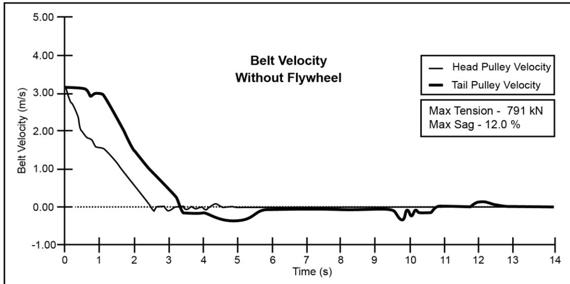
Figure 3. Belt speed without flywheels (emergency stop) [5]
