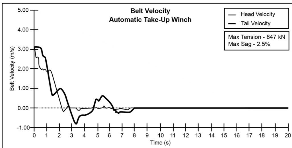
Figure 5. Belt speed with an automatic take-up winch (emergency stop) [5]
