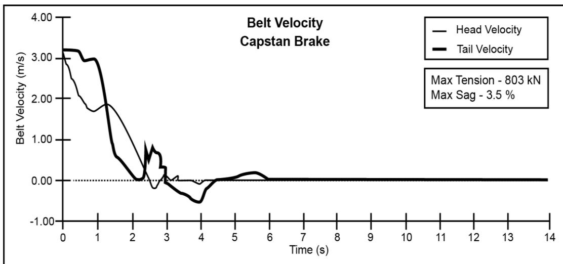
Figure 6. Belt speed with a capstan brake (emergency stop) [5]
