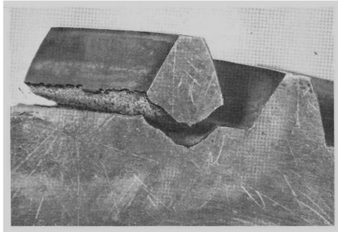
Figure 3. Bending fatigue failure <sup>2</sup>
