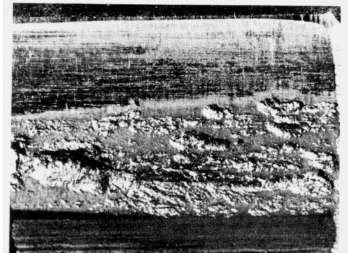
Figure 2. Pitted gear tooth <sup>2</sup>
