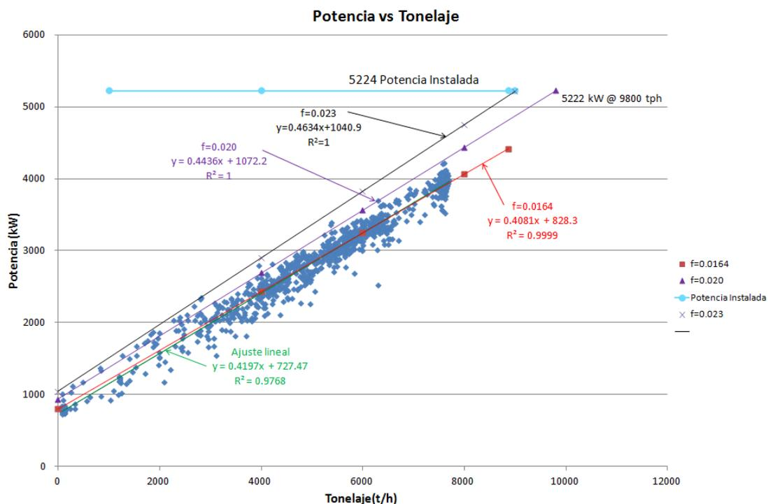
Figure 5. Overland conveyor field-measured and calculated power draw
