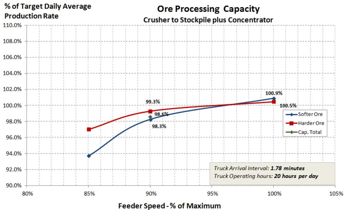
Figure 8. Complete crusher system and concentrator plant model results
