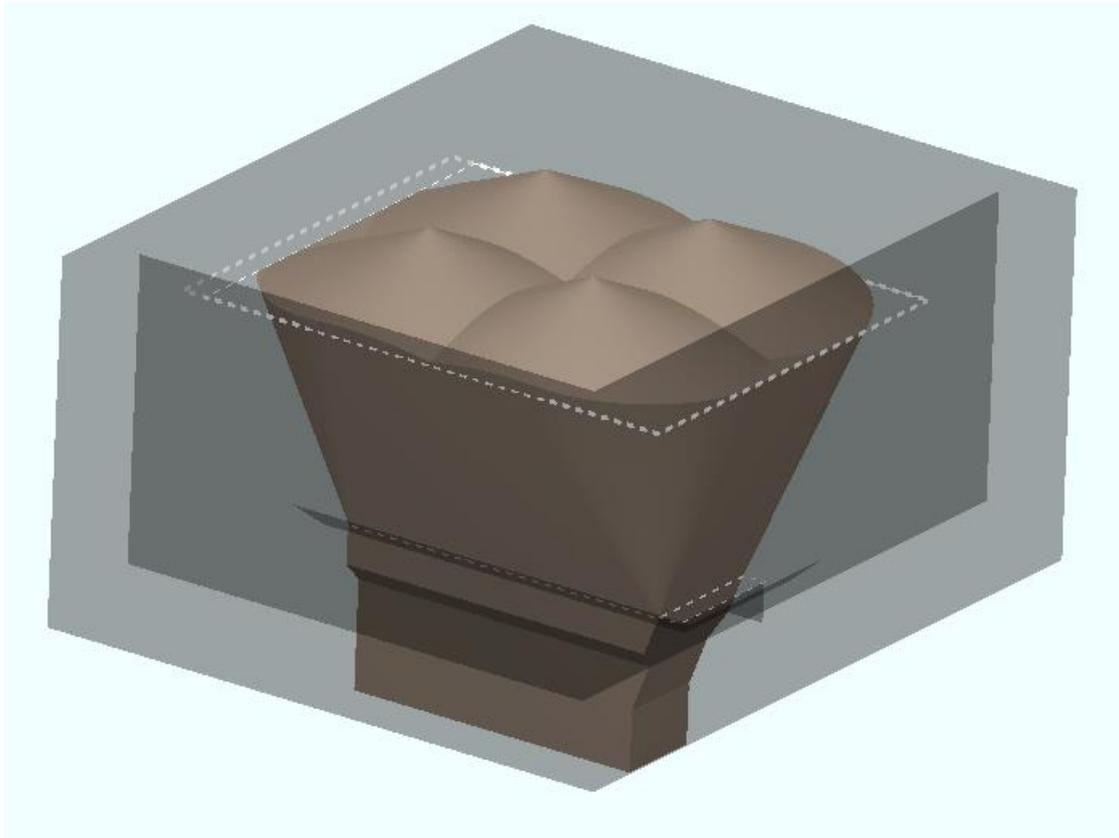
Figure 2. 3D view of typical surge bin live capacity
