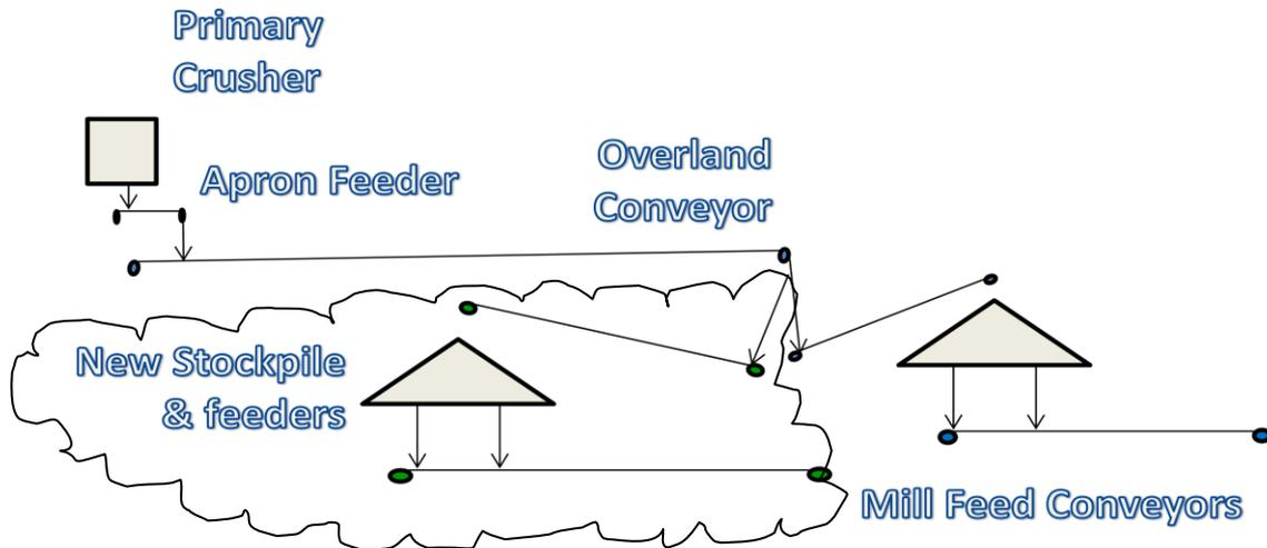
Figure 1. Schematic – Ore crushing and coarse ore conveying system upgrade
