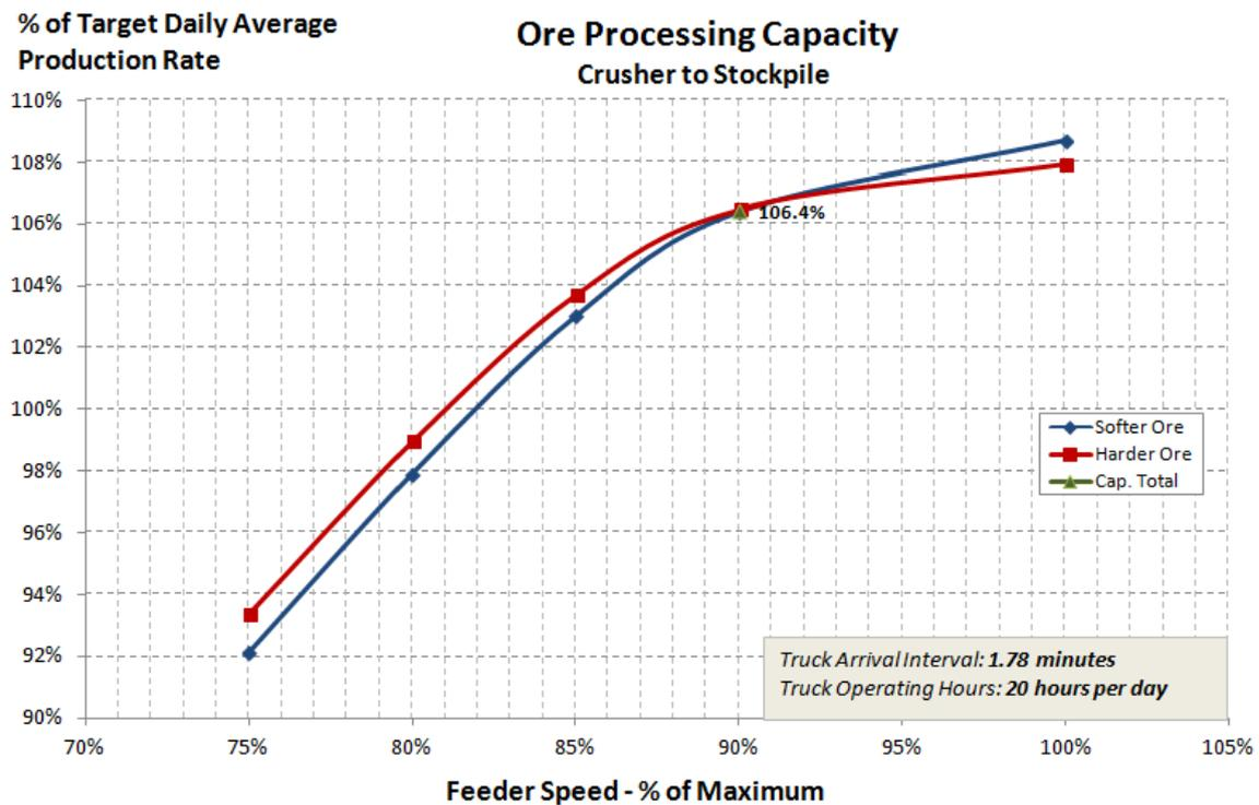
Figure 6. Crusher system model results
