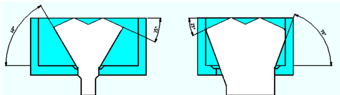
Figure 3. Typical surge bin live capacity geometry
