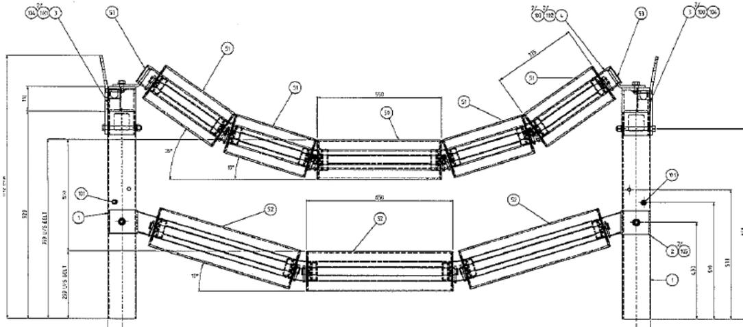
Figure 7. Type 1 idler configuration on stockyard conveyor
