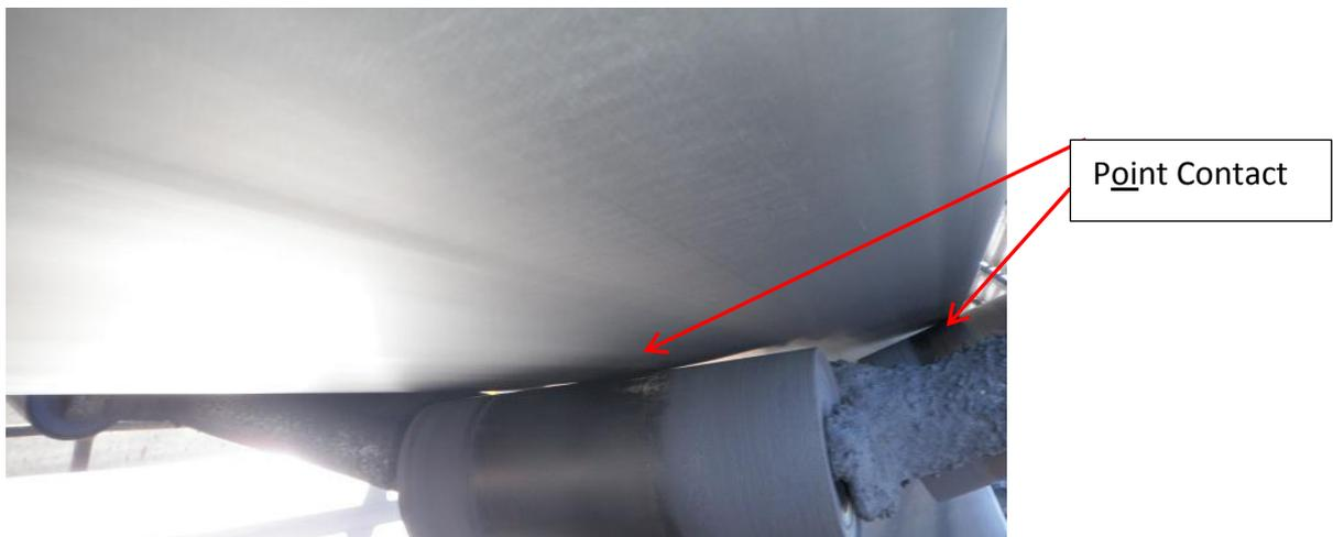
Figure 8. Type 1 belt contact with the idlers
