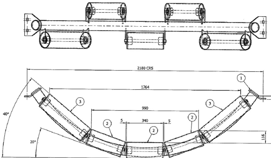
Figure 9. Type 2 idler configuration on stockyard conveyor
