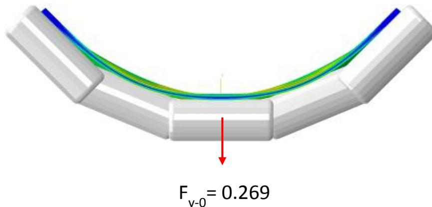
Figure 2. Five-roll 45° idler configurations
