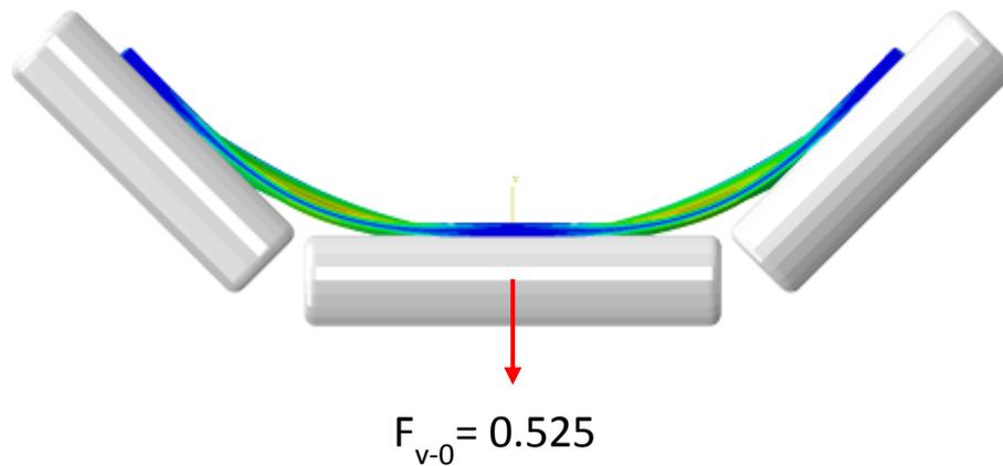
Figure 1. Three-roll 45° idler configurations
