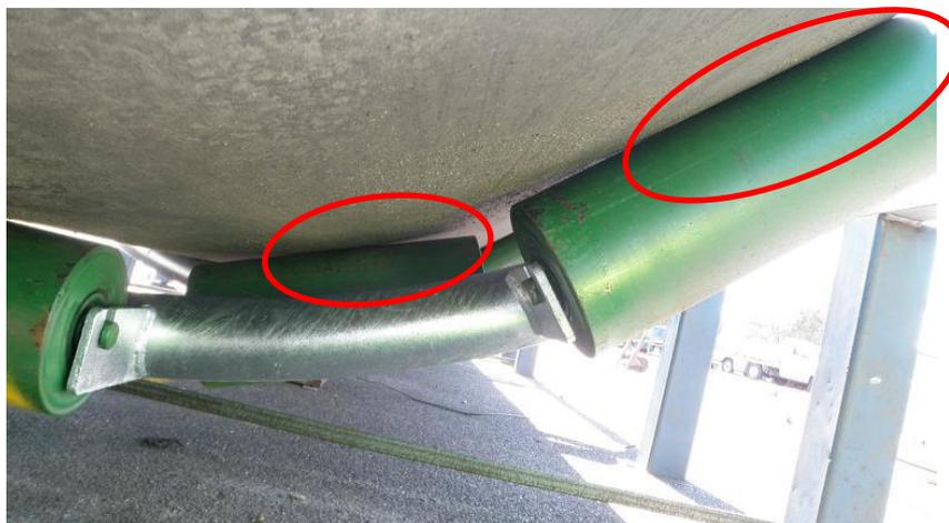
Figure 10. Type 2 belt contact with idlers
