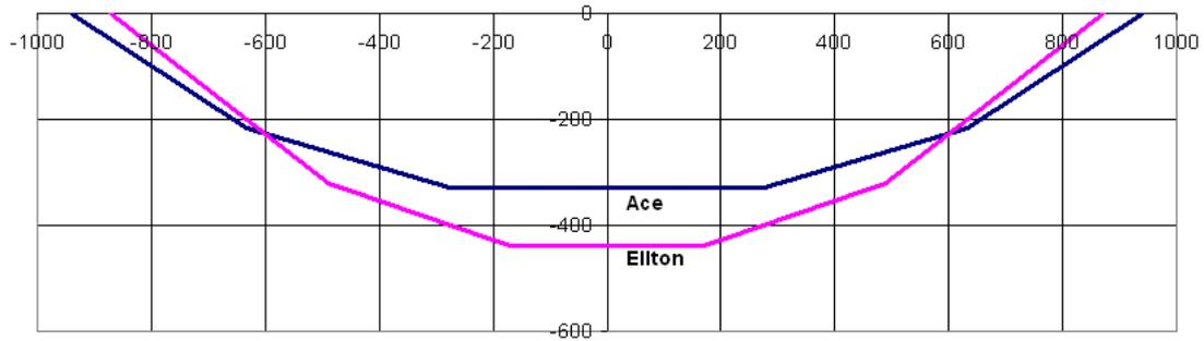
Figure 3. Chart showing different five-roll idler profiles
