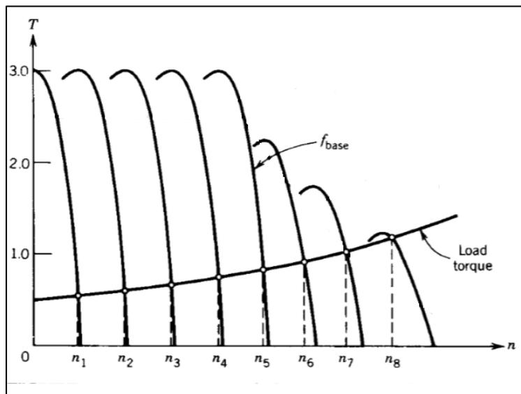
Figure 2. VVVF torque vs speed curves<sup>1</sup>
