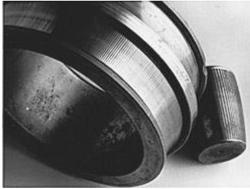
Figure 8. Bearing fluting<sup>6</sup>
