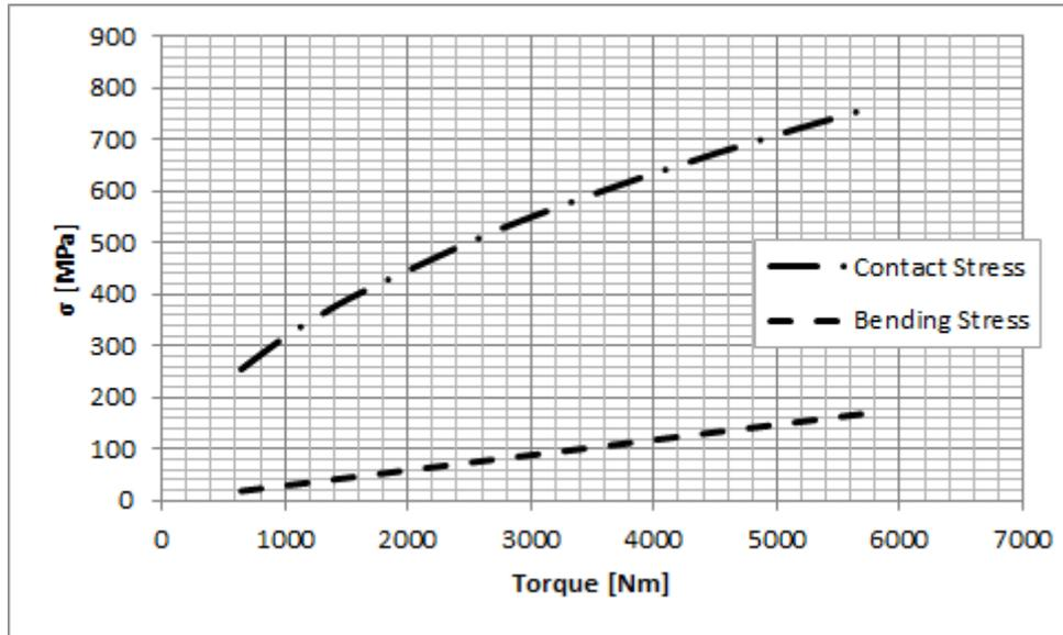
Figure 4. Gear teeth stress with torque
