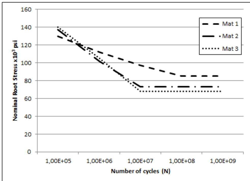
Figure 3. Fatigue life of low alloy carburised gears with nominal stress <sup>2</sup>
