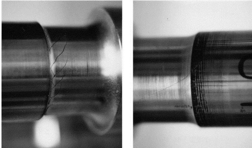
Figure 4. Oscillating torque induced fatigue shaft failures<sup>4</sup>
