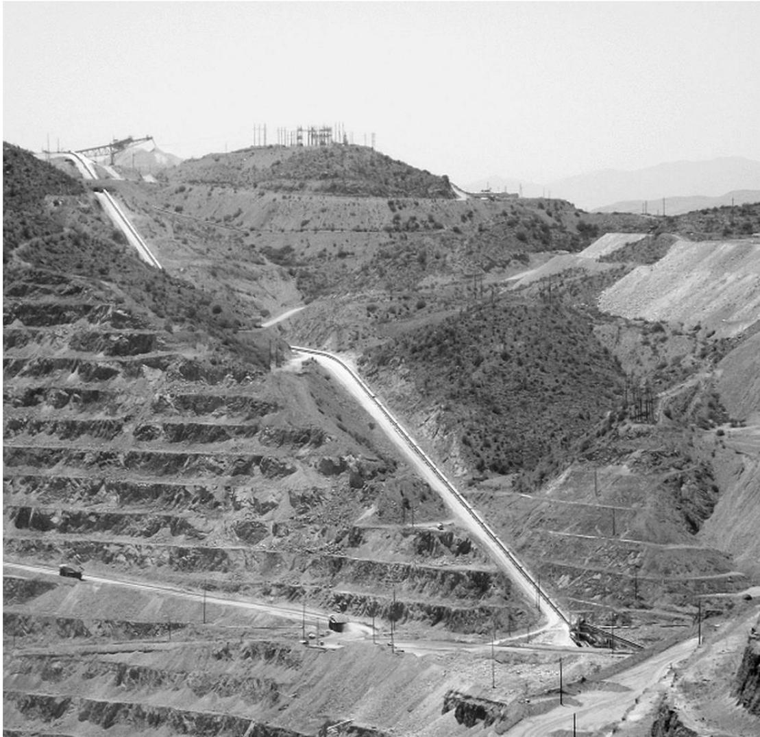
Figure 5. Ramp conveyor at a copper mine, Arizona. The difference in inclination between a truck ramp and an IPCC conveying ramp is clearly visible
