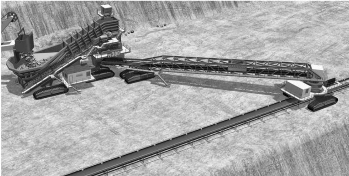
Figure 3. PF300 fully mobile crushing system consisting of a loading shovel, the mobile crusher, a belt bridge and a track-shiftable bench conveyor
