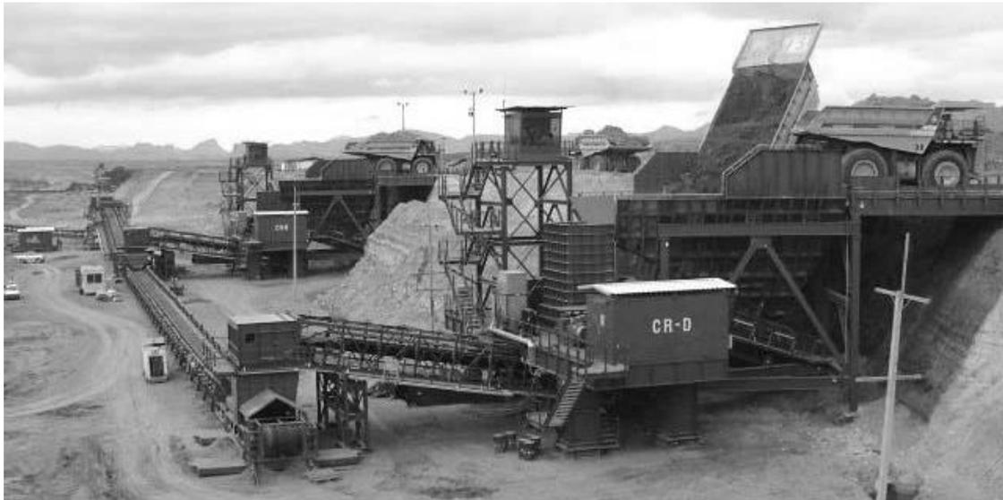
Figure 2. Semi-mobile crushers feeding one overland conveyor
