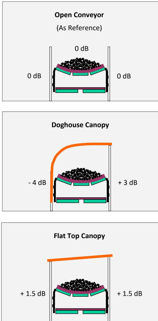
Figure 3. Typical directional characteristics of conventional conveyor canopies
