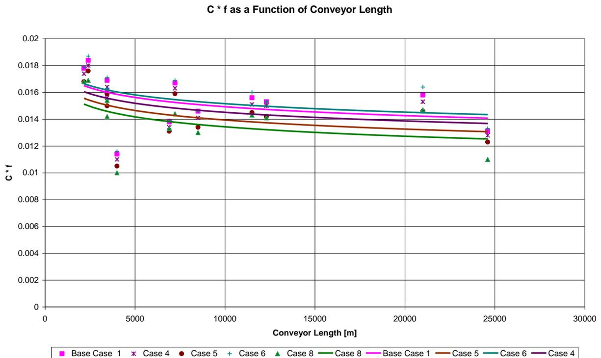
Figure 5. Values of C\*f as a function of conveyor length. Grade M cover (Base Case 1), increased central trough roll diameter (Case 4), increased trough rolls diameter (Case 5), unequal trough rolls length (Case 6), low resistant idlers (Case 8).
