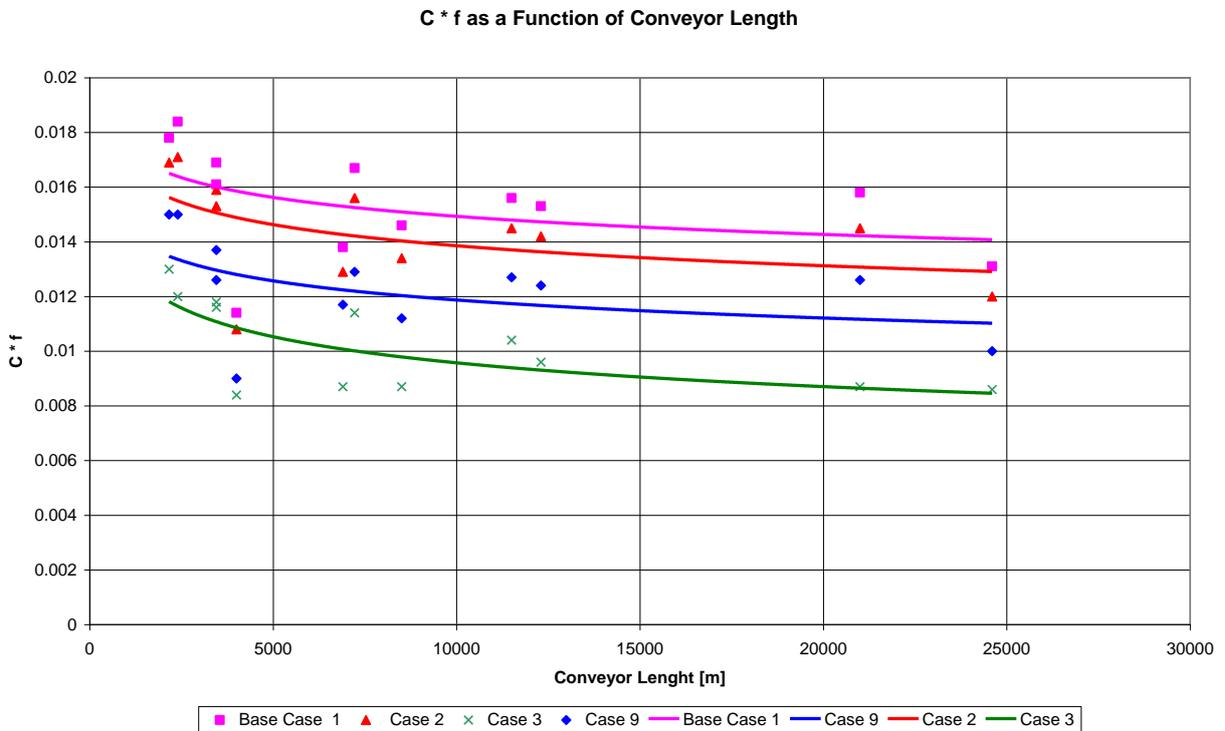
Figure 7. Values of C\*f as a function of conveyor length. Grade M cover (Base Case 1), LRR cover (Case 2), Special LRR cover (Case 3), combined LRR cover, increased trough roll diameter, low resistance idlers (Case 8)
