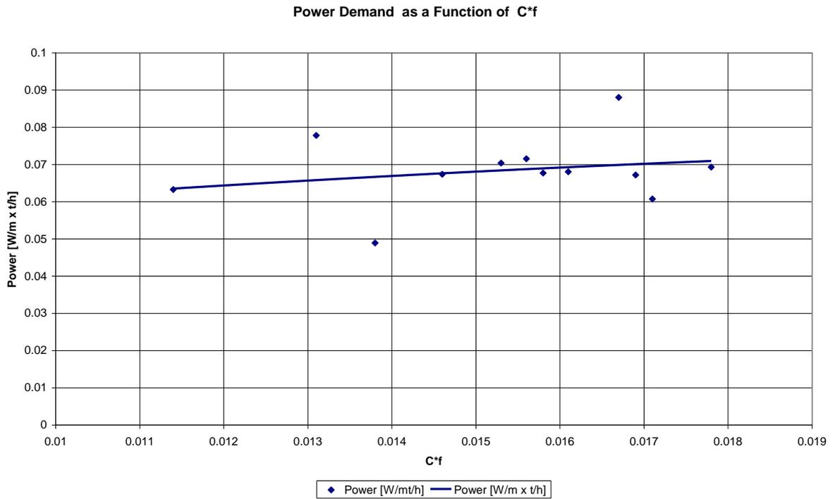
Figure 13. Conveyor unit power demand as a function of C\*f (Base Case 1).
