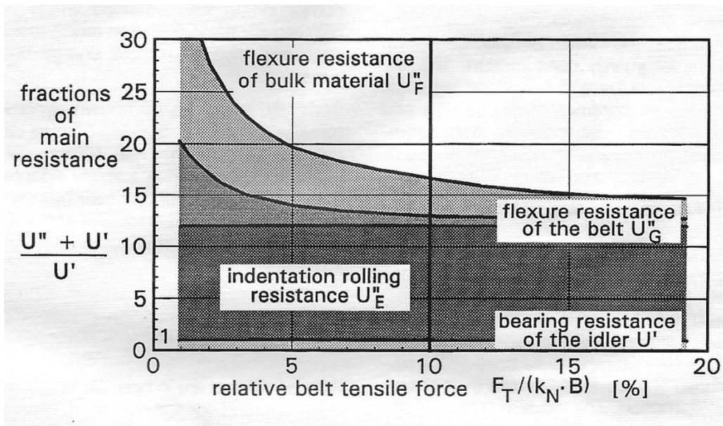
Figure 1. Influence of belt tension on the individual main resistances with respect to the bearing resistance of the idlers.  $F_T$  – belt tension [kN];  $k_N$  – ultimate belt tension [kN/m];  $B$  – belt width [m]
