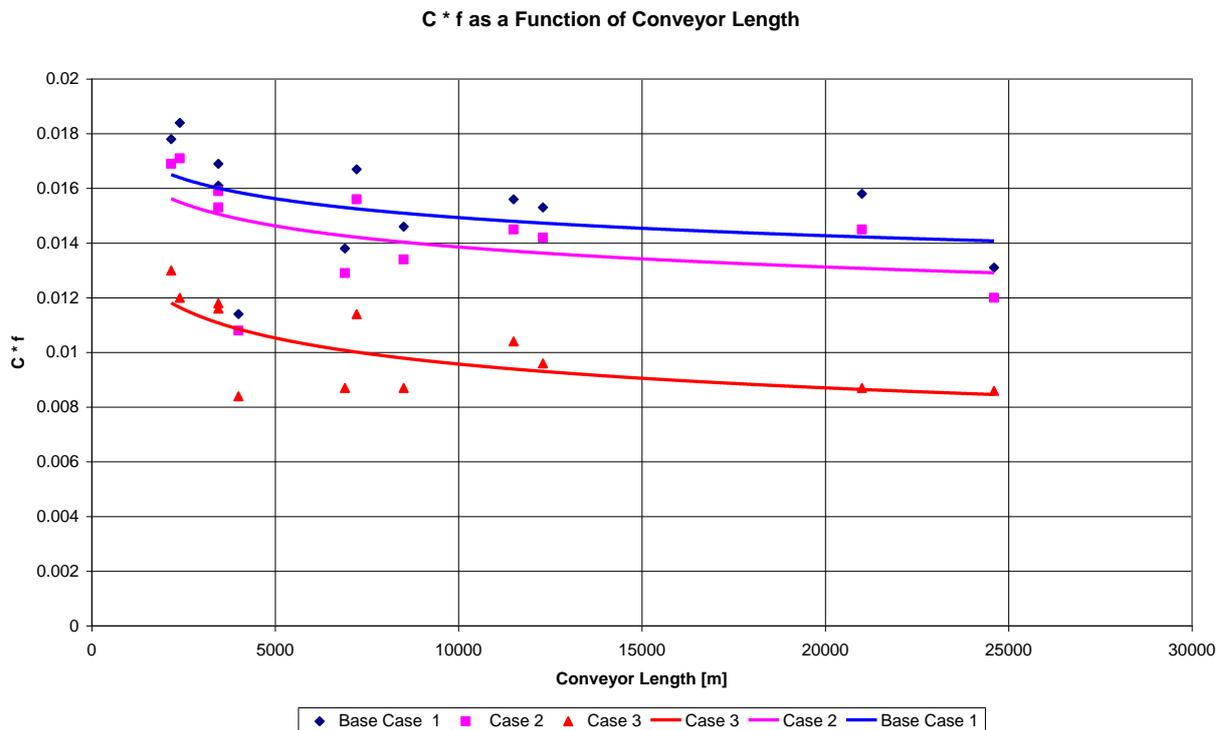
Figure 4. Values of C\*f as a function of conveyor length. Grade M cover ( Base Case 1), LRR cover (Case 2) and Special LRR cover (Case 3)
