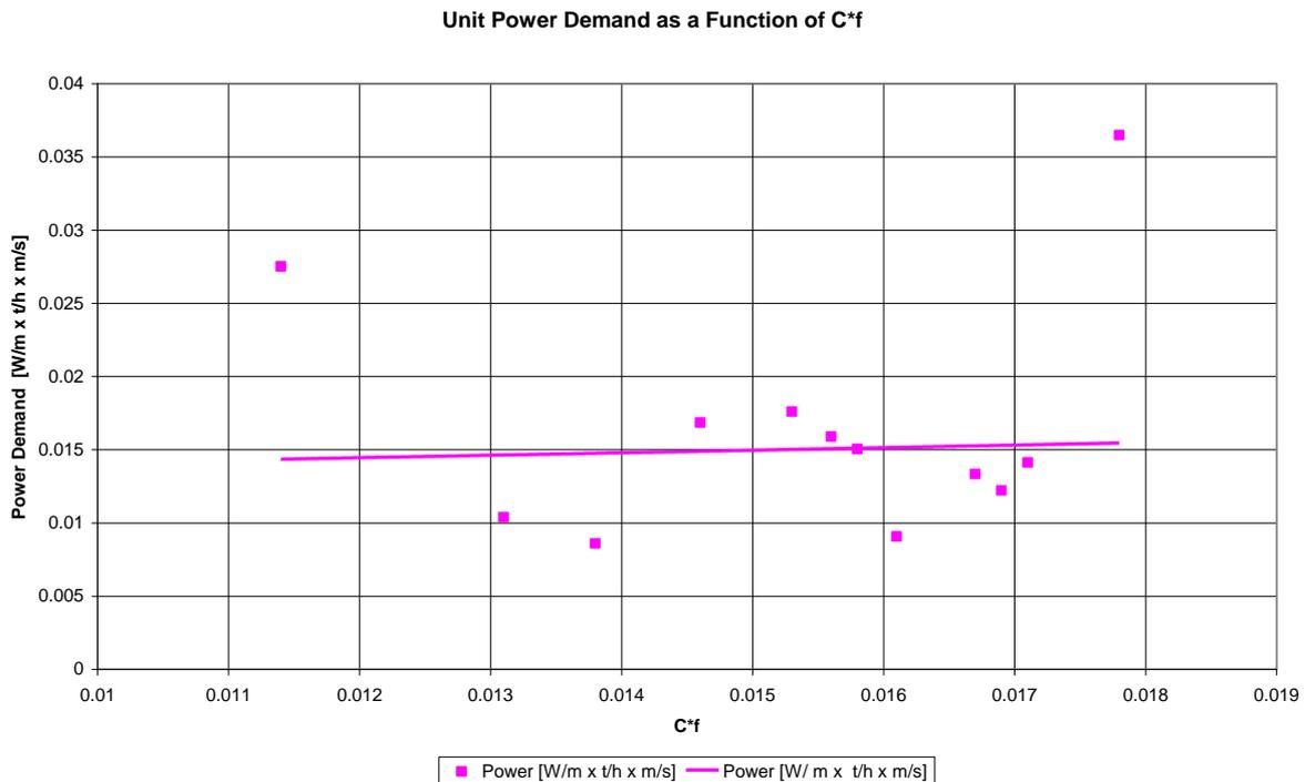
Figure 12. Conveyor unit power demand as a function of  $C \cdot f$  (Base Case 1).
