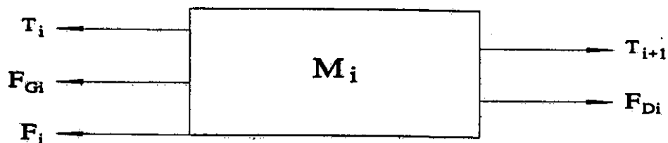
Figure 5. A single conveyor element used for the discrete model.
