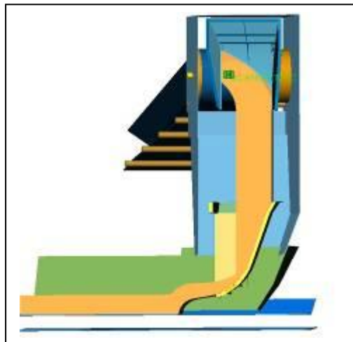
Figure 9 ~ Confirmation of material flow characteristics through cross sectional views of material flow
