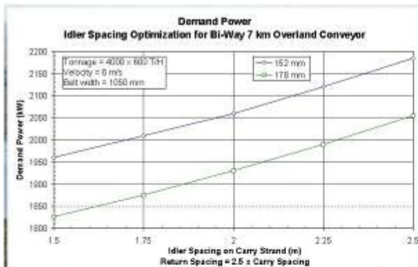
Fig. 7b Demand Power vs Idler Spacing & Roll Diameter
