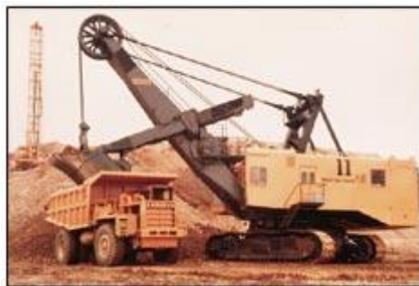
Fig.3 Electric Shovel and Trucks
