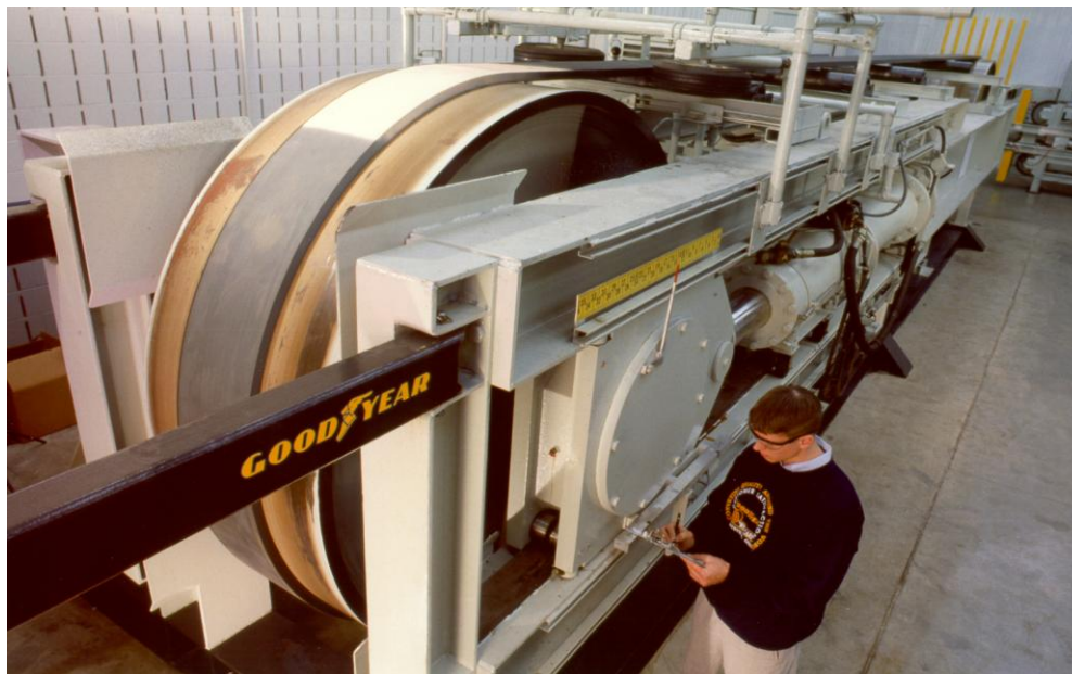
Fig.23 2-Pulley Dynamic Splice Test Machine, in the manufacturer's Technical Center
