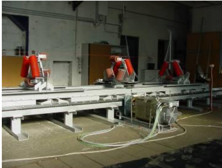
Figure 8: The measuring slide with drive motor and steering rack
