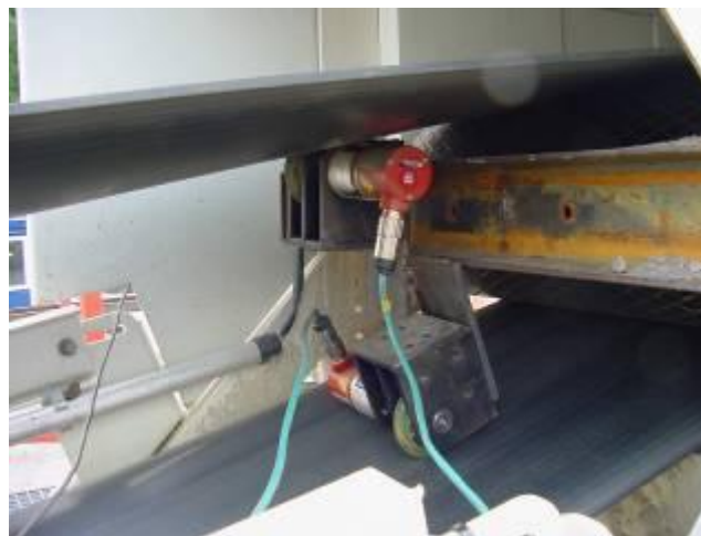
Figure 14. Measurement of belt tension in carry side and return side
