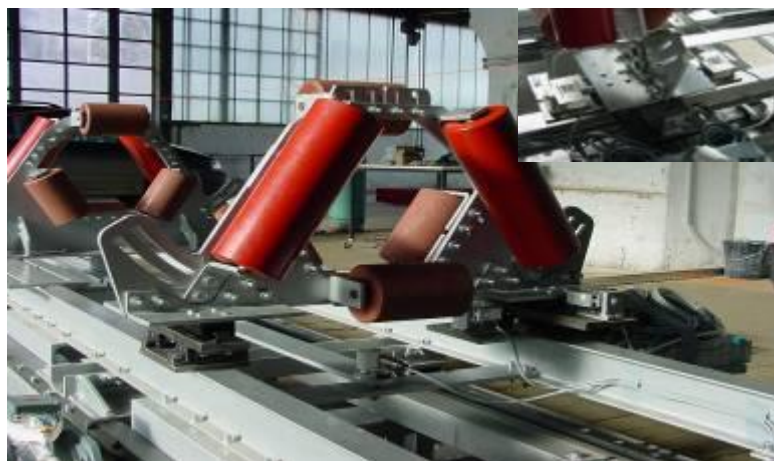
Figure 7: The measuring idler station on the measuring slide
