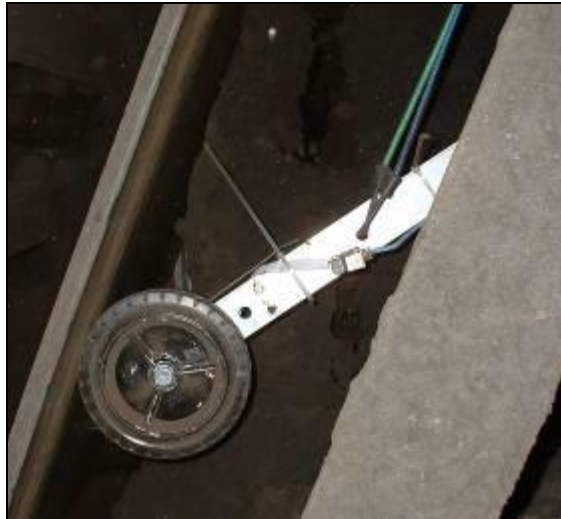
Figure 7: Simple velocity measurement using an optical encoder and measurement wheel
