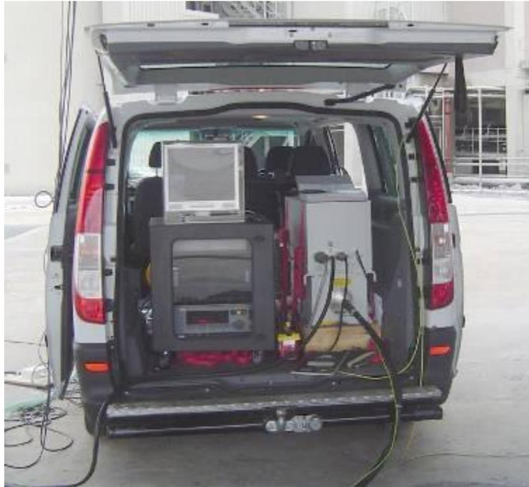
**Figure 1:** The X-ray survey vehicle containing the DiXI system.
