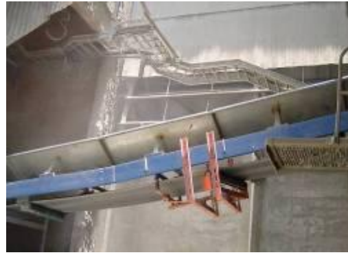
FIGURE 9 Modular Sections of the Conveyor were Mitered to Accommodate the Vertical Curve.
