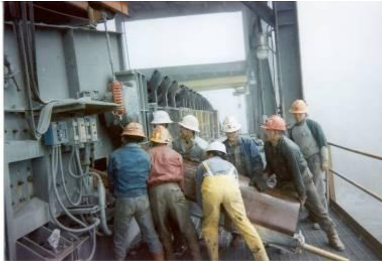
FIGURE 10 Developed For Applications in Open Pit Lignite Mines, the Super Heavy-Duty Belt Cleaner Features Massive Blades on a Steel I-Beam Frame
