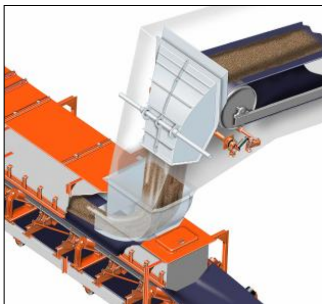
FIGURE 1 Engineered Flow Chutes Typically Include a “Hood” (Top) to Direct the Material Flow and a “Spoon” (Bottom) to Place the Material on the Receiving Belt
