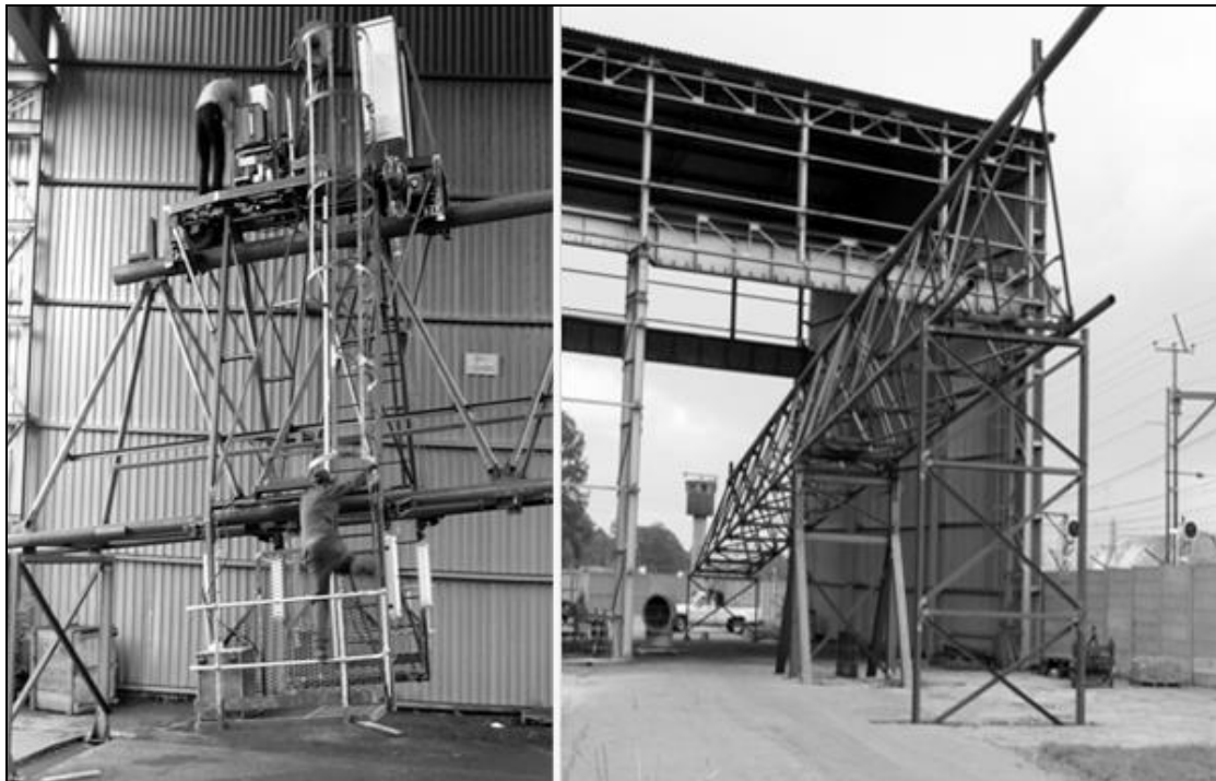
Figure 10 – Trolley test installation on elevated gantry
