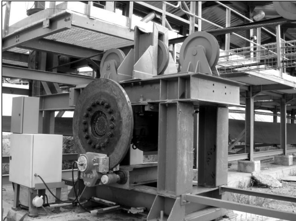
Figure 5 – Capstan brake between the counterweight mass and take-up pulley
