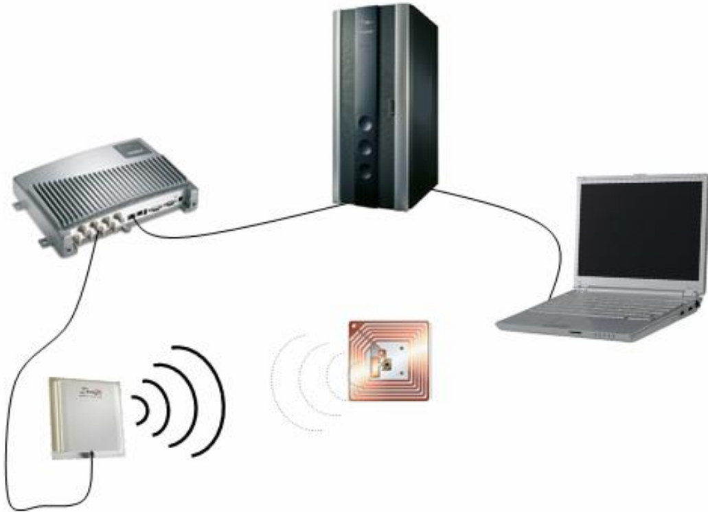
Figure 2: Components of an RFID system.
