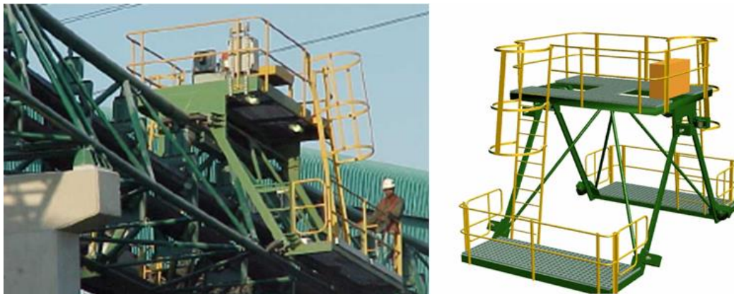
Figure 1: Maintenance trolley installed on the RBCT terminal in Richards Bay, Republic of South Africa [courtesy CKIT].
