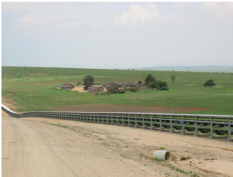
Figure 6: Large scale overland belt conveyor in South Africa (courtesy Conveyor Experts B.V.).
