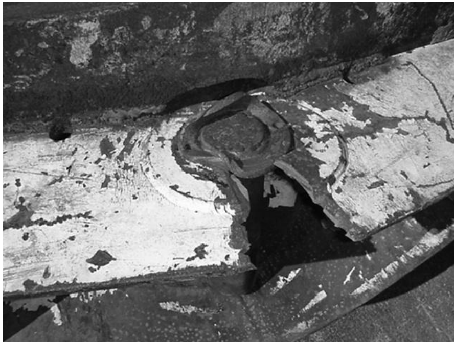
Structural Failure as a Result of Rapid Belt Contraction
