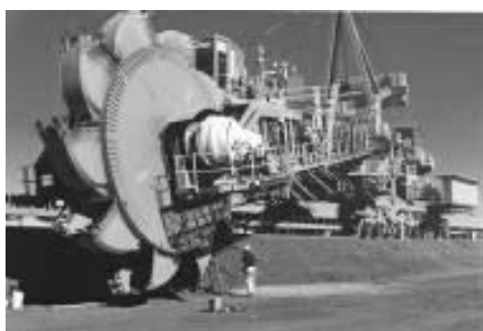
Fig 1: A Bucket Wheel is a typical low speed drive application
