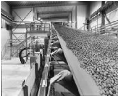
Fig 20: 1575 Kw drive on the 8500 Tph inclined conveyor
