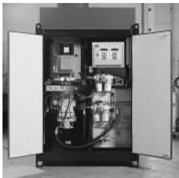
Fig 6: A power unit supplies fluid to the hydraulic motor
