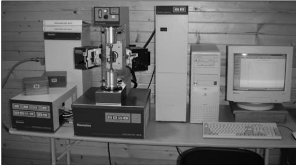
Figure 10 –Rubber rheology instrument used to determine belt cover properties
