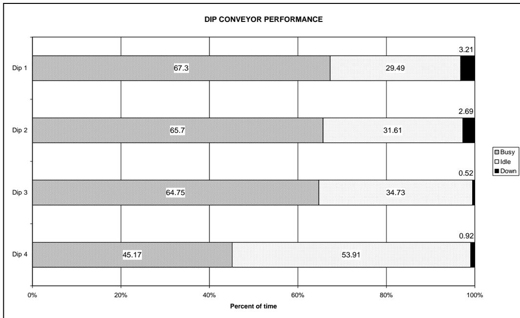
Fig 10: Example of decline conveyor utilisation
