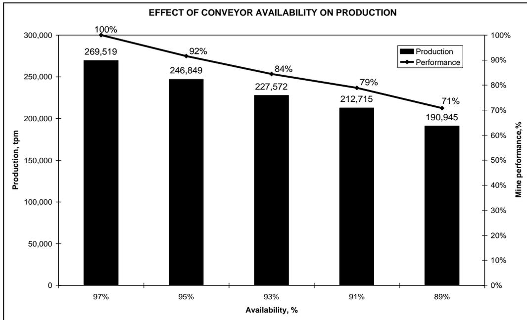
Fig 11: Effect of conveyor availability on mine performance
