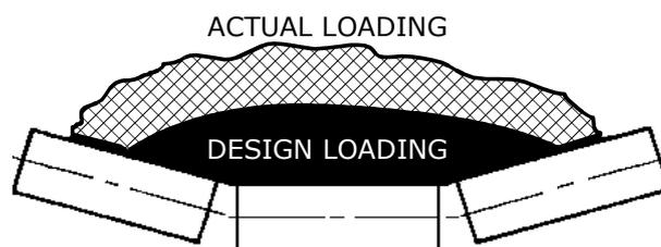
Fig 4: Actual versus design volumetric loading
