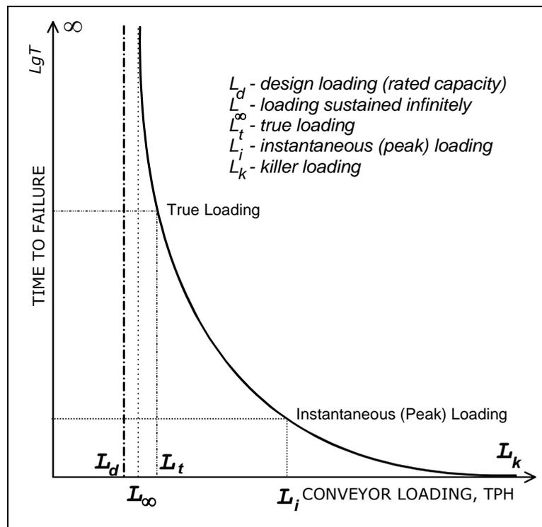
Fig 9: Illustrative correlation between conveyor loading and time it can be sustained (time to failure)
