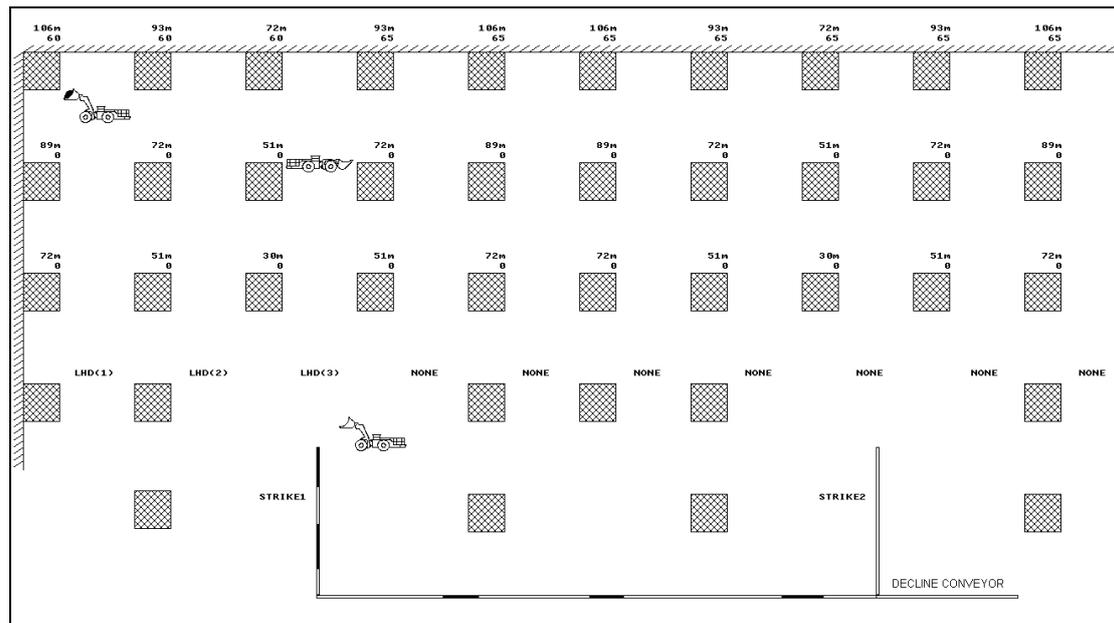
Fig 5: Discrete flow of material on conveyors loaded with LHD direct tipping
