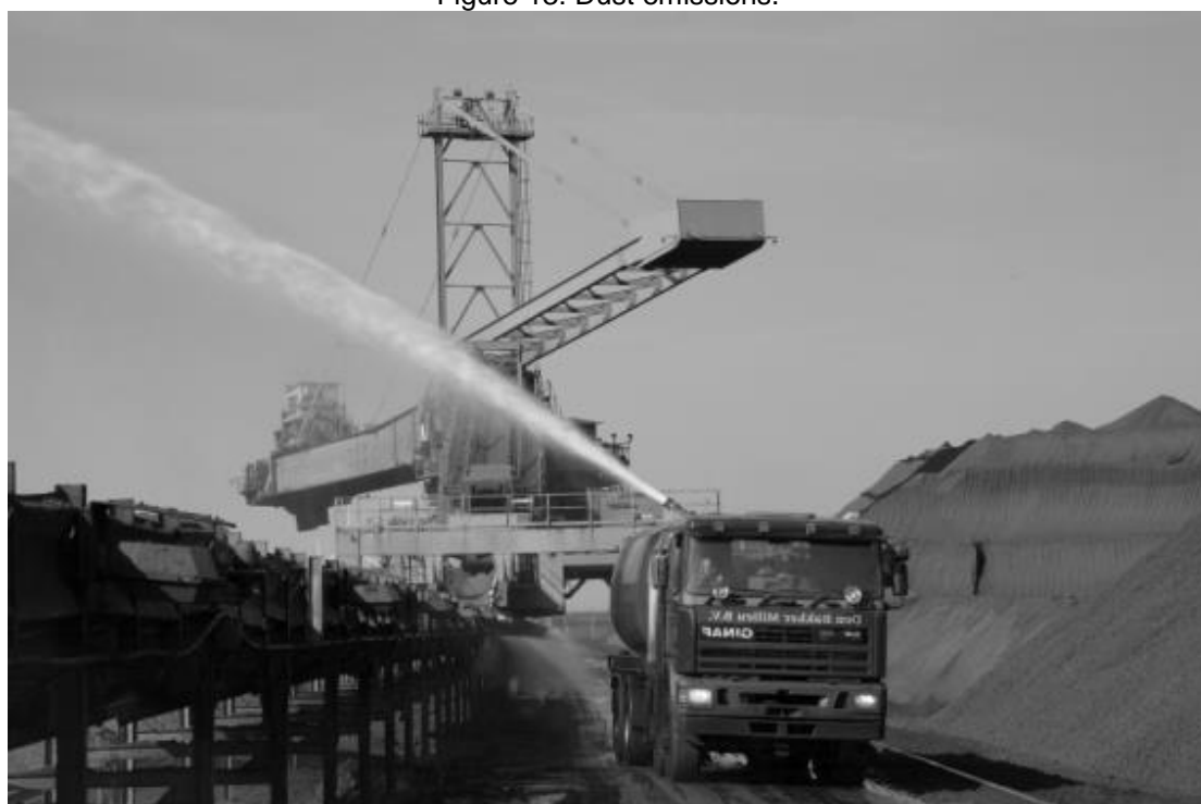
Figure 14: Environmental protective measures at a Dutch bulk terminal.
