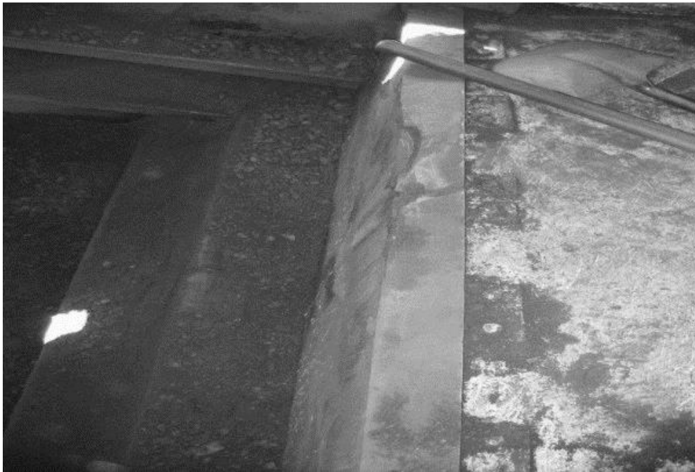
Figure 5.6 – Wear on high capacity chute
