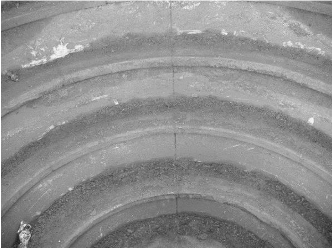
Figure 5.5 – Wear on high capacity chute allowing material flow routes to be clearly demarcated to allow flow analysis
