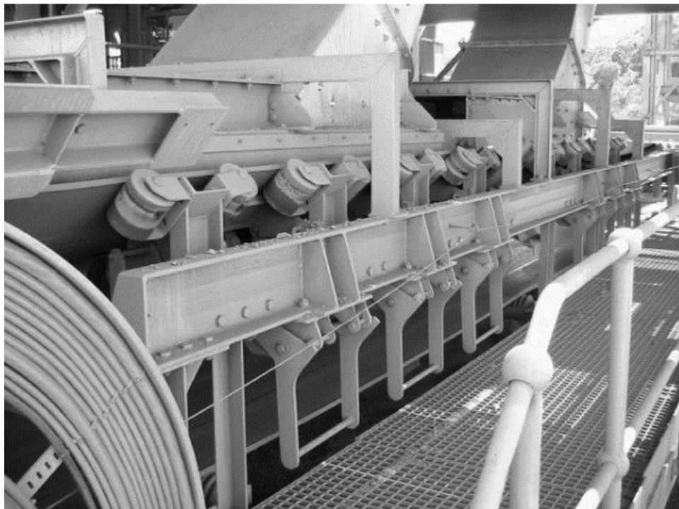
Figure 7.2 – Typical impact arrangement
