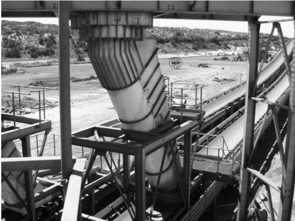
Figure 4.1 – Typical Multi Product Transfer Chute
