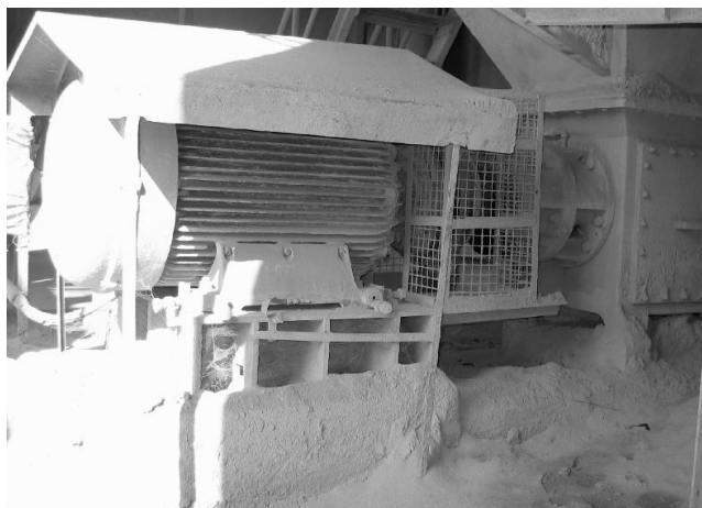
Figure 5: Typical Dust Likely to Contaminate Machinery Elements
