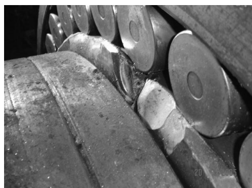
Figure 10: Converter Bearing – Detected at 1.5 rpm
