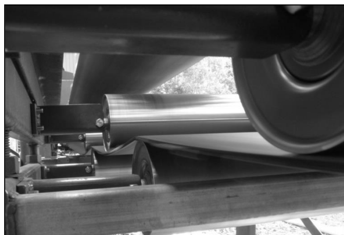
Figure 9. Zigzag path of conveyor belt through test rig
