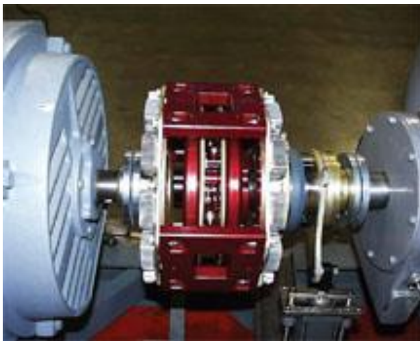
Figure 9. Adjustable speed drive installation with actuator
