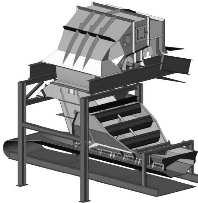
Figure 19. Shiploader 3, elevator to boom CAD Image
