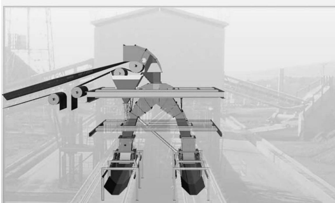
Figure 12. Typical reclaim conveyor to Shipping streams 1 and 2 yard conveyors, chute details
