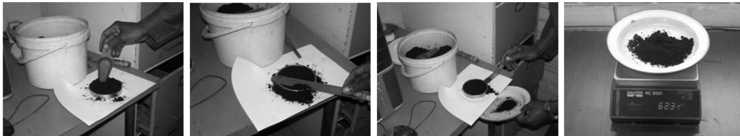
Figure 15. Bulk density test procedure
