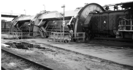
Figure 10. Wagons being tipped (tippler side view)
