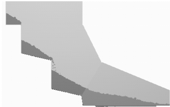
Figure 20. Side view of DEM prediction of the material profile of dry bauxite with no material flow in lower chute section
