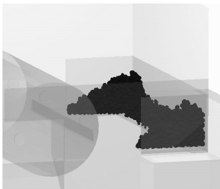
Figure 17. DEM prediction of the material profile of wet bauxite with no material flow in the upper head chute
