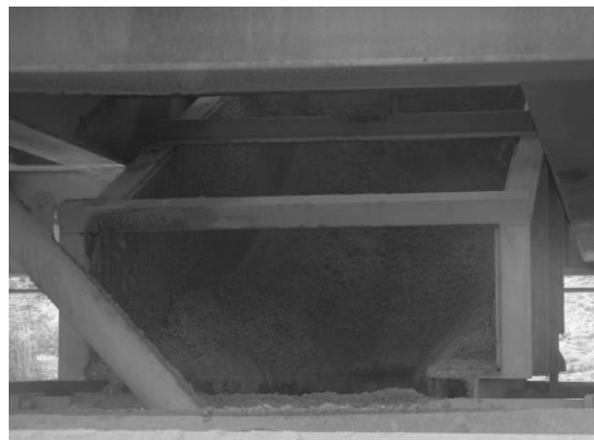
Figure 22. Front view of the material profile of wet bauxite with no material flow in the feed chute
