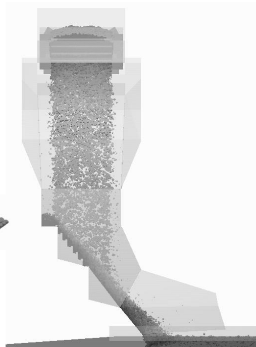
Figure 33. Side view of DEM simulation of Concept B with upper impact plate
