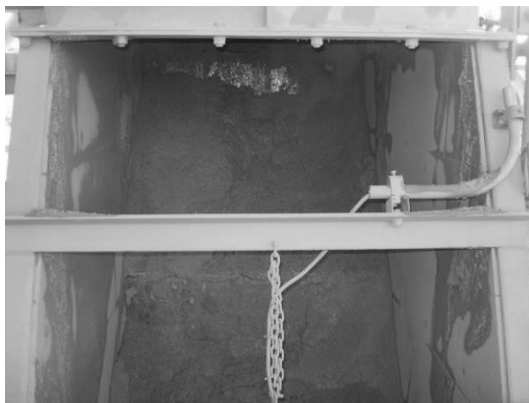
Figure 21. Front view of the material profile of wet bauxite with no material flow in the rock box
