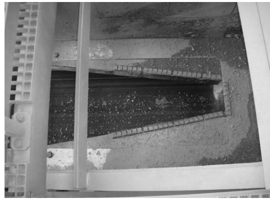
d) V-Plate in feed chute restricting flow
