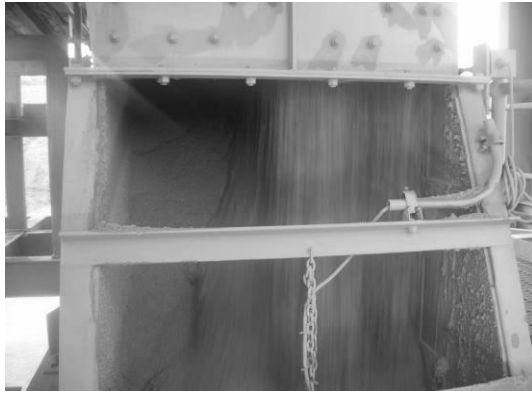
a) Non-symmetrical flow in the lower section of the chute
