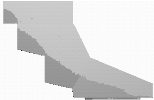
Figure 19. Side view of DEM prediction of the material profile of wet bauxite with no material flow in lower chute section
