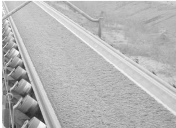
Figure 14. Profile of wet bauxite on C2
