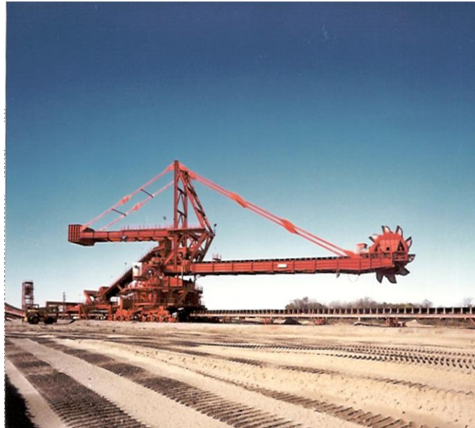
Figure 3. Bucket wheel reclaimer (single point reclamation)
