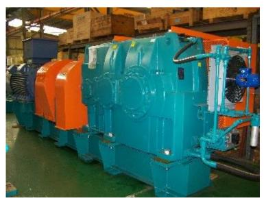
Figure 1. Belt conveyor drive with flywheel (courtesy Hansen)
