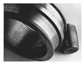
Figure 8. Bearing fluting<sup>6</sup>
