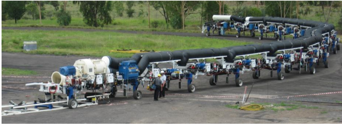
Figure 9. Prairie Flexiveyor undergoing surface commissioning at an Australian colliery (Prairie, N.D.)
