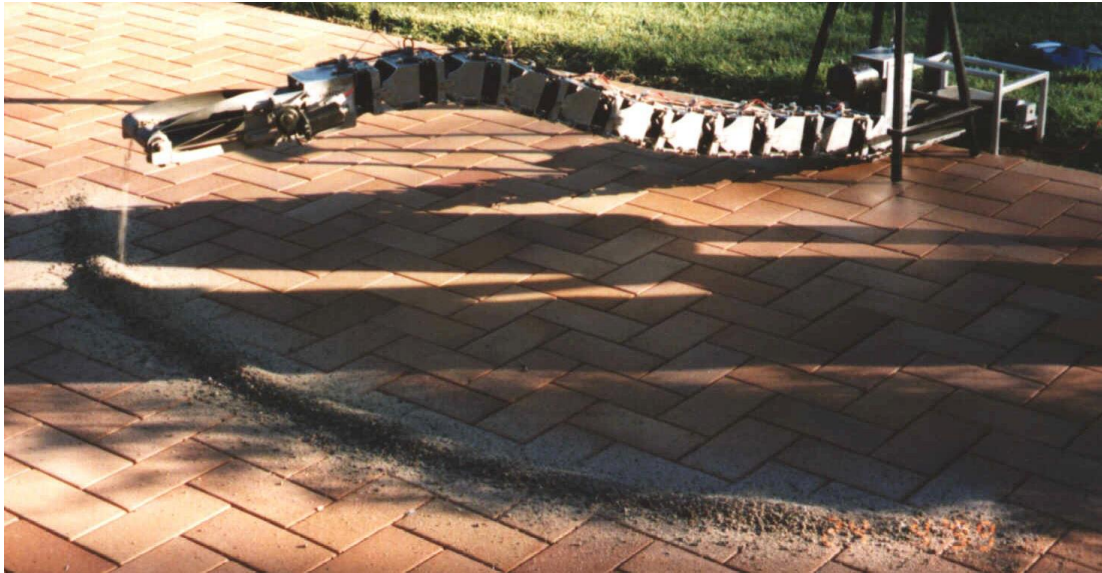
Figure 3. Working laboratory scale-model of Bosmin Co-axial Pipe Conveyor (Bosmin, N.D.)
