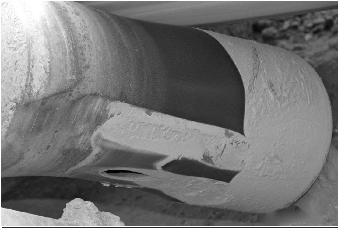
Figure 9. Worn and seized idlers
