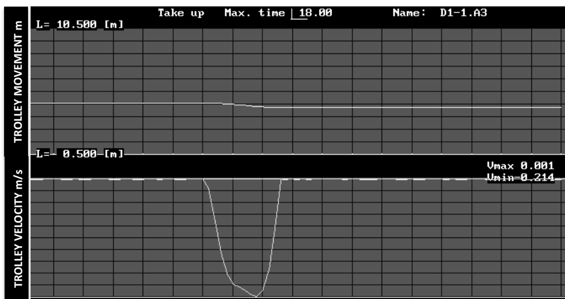
Figure 26. Winch inactive, overload protection (slip clutch) installed. Graphs of take-up trolley movement [m] (upper) and take-up trolley velocity [m/s] (lower)
