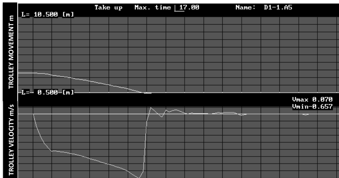
Figure 28. Winch inactive, overload protection (slip clutch) installed – set at 68.5 kN. Graphs of take-up trolley movement [m] (upper) and take-up trolley velocity [m/s] (lower)
