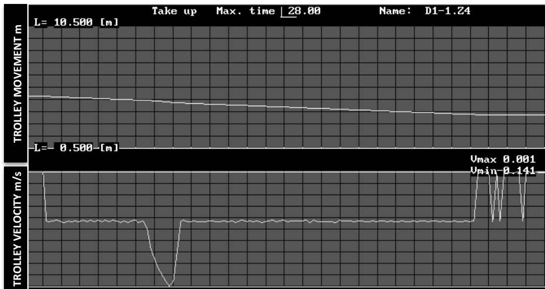
Figure 12. Winch active DOL – constant speed winch operation, overload protection (slip clutch) installed – set at 137 kN. Graphs of take-up trolley movement [m] (upper) and take-up trolley velocity [m/s] (lower)
