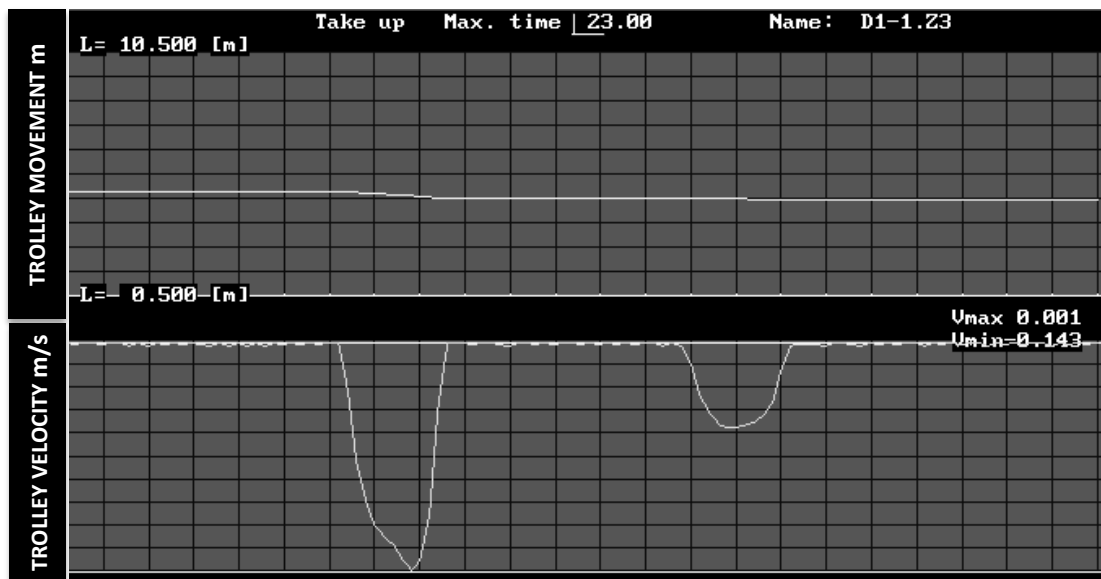
Figure 8. Winch inactive, overload protection (slip clutch) installed. Graphs of take-up trolley movement [m] (upper) and take-up trolley velocity [m/s] (lower)
