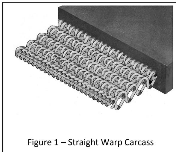
Figure 1 – Straight Warp Carcass
