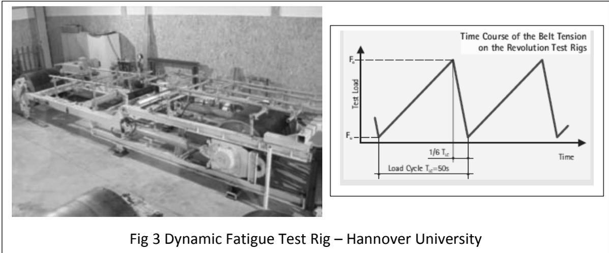
After searching test records for textile reinforced belts joined by finger splices it was found that dynamic tests of high strength solid woven finger splices returned an efficiency of just over 30% on the dynamic fatigue splice test rig at Hannover University.
