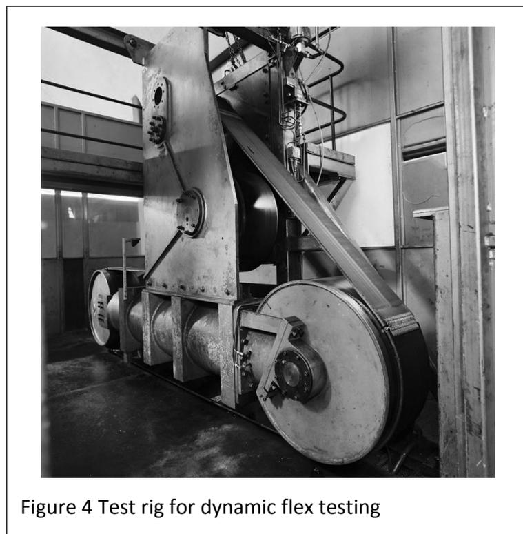
12.5% of breaking strength and increasing by 5% every 125000 cycles until the belt failed. Belts all failed at the splice during the load cycle of 27 to 32% of whole belt breaking load. Thereafter the tensile strength of the belt was measured. A reduction of less than 5% in strength indicated that the belt construction can be subjected to high tension in reverse bending applications without any detrimental effects.
