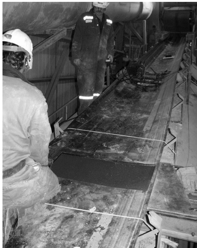
Figure 6. Retrofitting of Sensor loop
