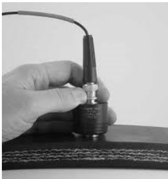
Figure 13. Handheld ultrasonic thickness measurement tool.
