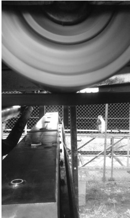
Figure 19. Sensor array fitted below calming idler
