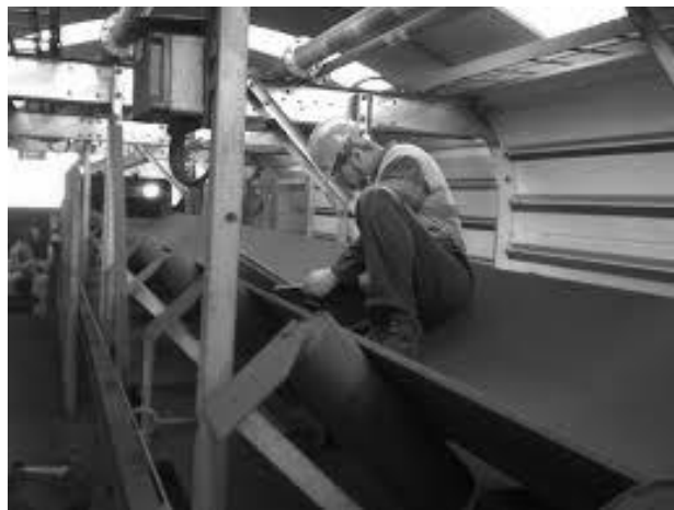
Figure 12. Measurement is done with handheld ultrasonic measuring equipment.
