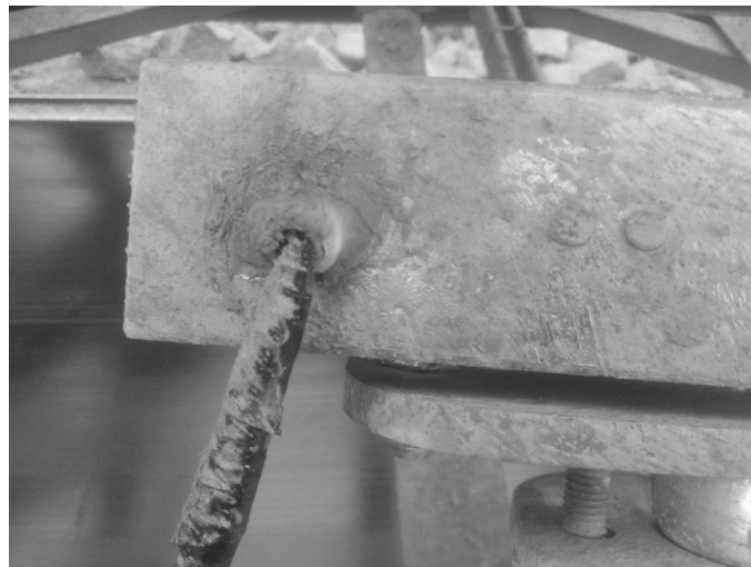
Figure 7. Damage to transmitter cable due to spillage
