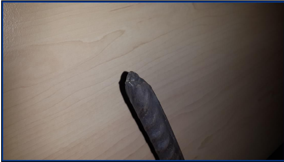
Figure 8. Typical tensile failure of rebar.
