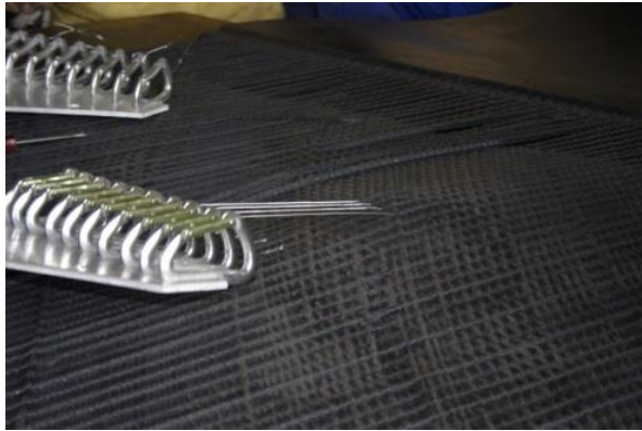
Figure 2. Piano wire steel cord stripper.
