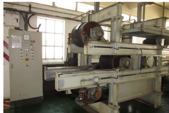
Figure 10. Conveyor system indicating positive and negative bends in short succession at pulleys A-C and at A-A.
