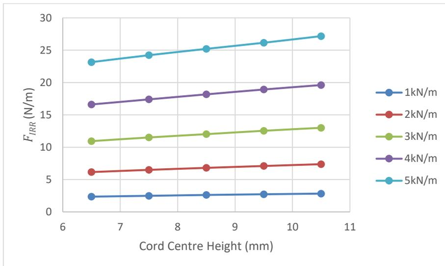
**Figure 0.7** Rearranged indentation rolling resistance simulation results versus different cord centre heights.
