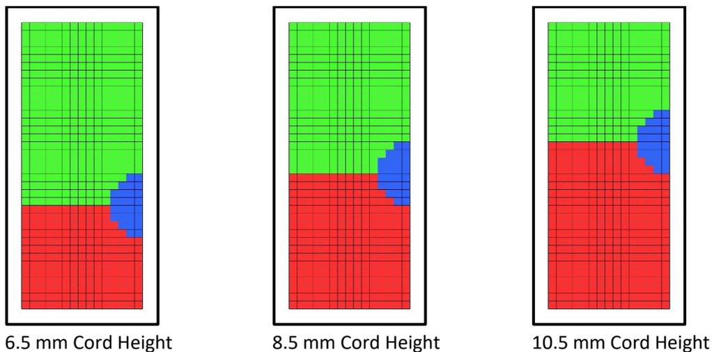
**Figure 0.5** Model cross sections for different cord centre heights.
