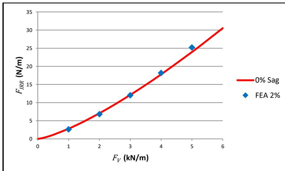
**Figure 0.4** A comparison of low rolling resistance conveyor belt 0% sag experimental and three dimensional simulation results.
