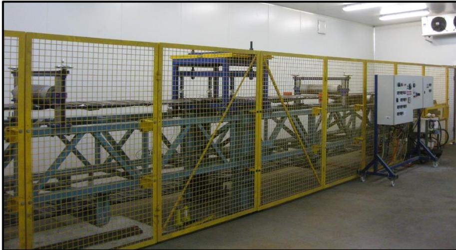
**Figure 0.3** The University of Newcastle’s large indentation rolling resistance test machine inside its temperature controlled room (Munzenberger, 2017)
