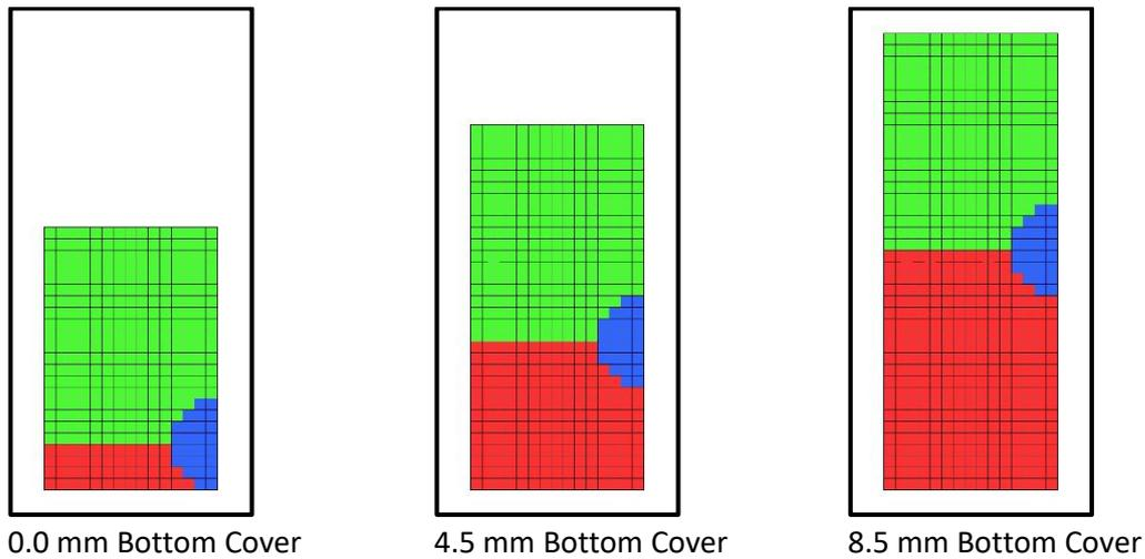
**Figure 0.15** Model cross sections for different bottom cover thicknesses
