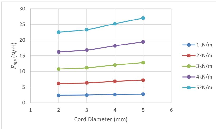
**Figure 0.11** Indentation rolling resistance results versus cord diameters for constant cord area models.
