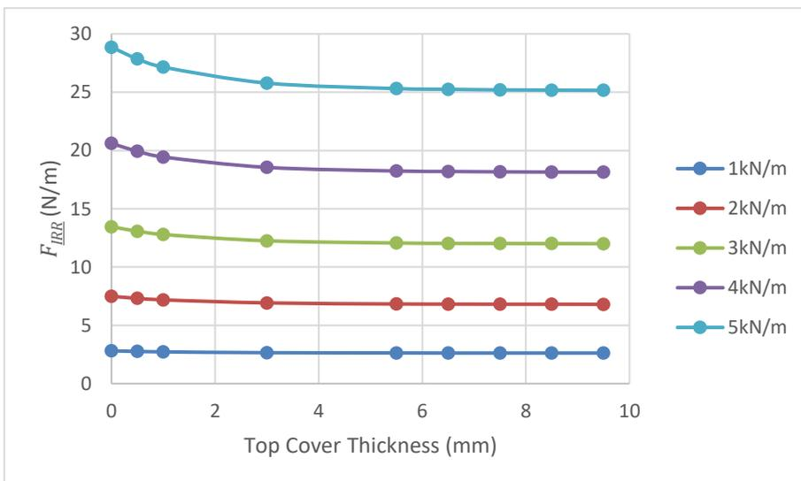
**Figure 0.20** Indentation rolling resistance results versus different top cover thicknesses
