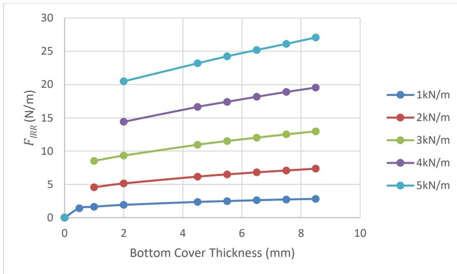
**Figure 0.17** Indentation rolling resistance results versus different bottom cover thickness
