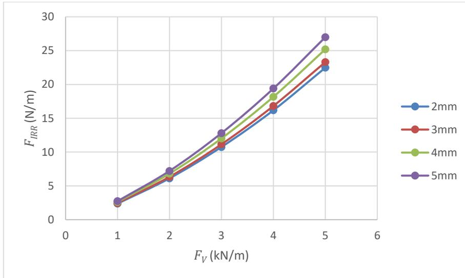
**Figure 0.10** Indentation rolling resistance simulation results for different cord diameters and constant cord area versus vertical load.
