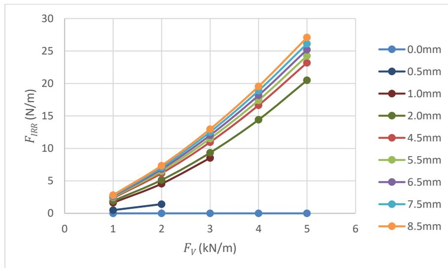
**Figure 0.16** Indentation rolling resistance predictions for different bottom cover thicknesses versus vertical load
