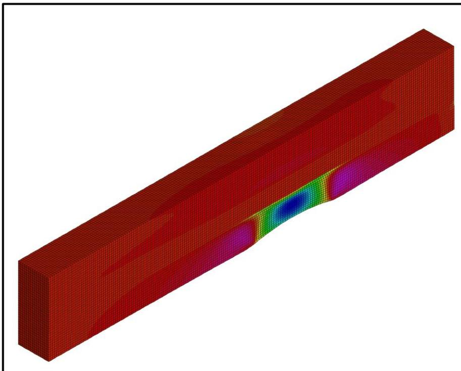
**Figure 0.2** The model from Figure 0.1 shown with strain contours superimposed on the elements
