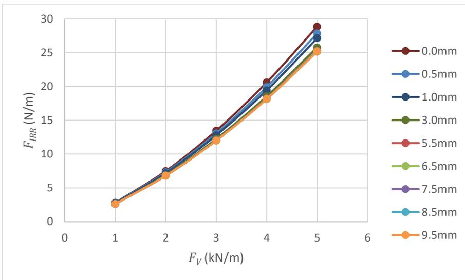
**Figure 0.19** Indentation rolling resistance simulation results for different top cover thicknesses versus vertical load
