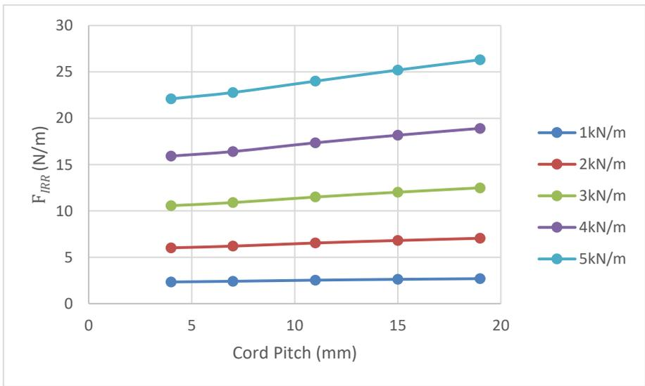
**Figure 0.14** Indentation rolling resistance results versus different cord pitch.
