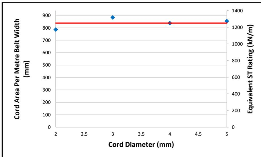
**Figure 0.9** Actual area of the conveyor belt model – per metre, marked by the line, and the actual areas achieved for each cord diameter modelled marked by the points. The two vertical axes scales are equivalent and relate to all graphed data.
