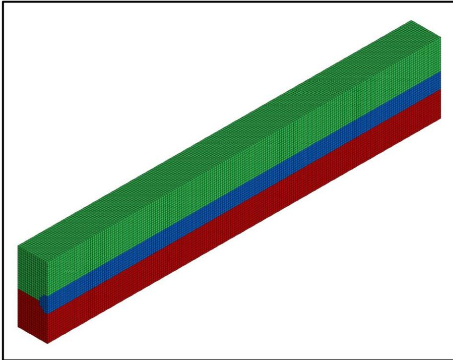
**Figure 0.1** A view of a three dimensional indentation rolling resistance model
