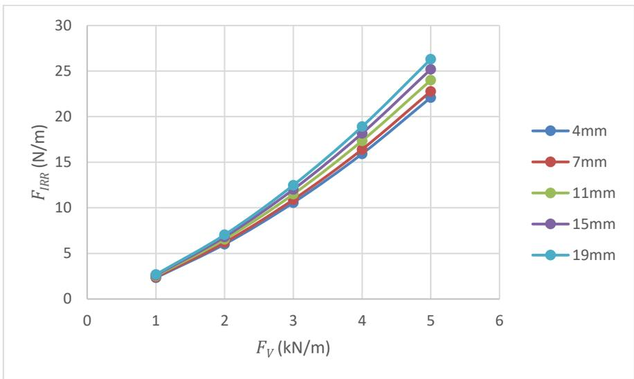
**Figure 0.13** Indentation rolling resistance simulation results for different cord pitches versus vertical load
