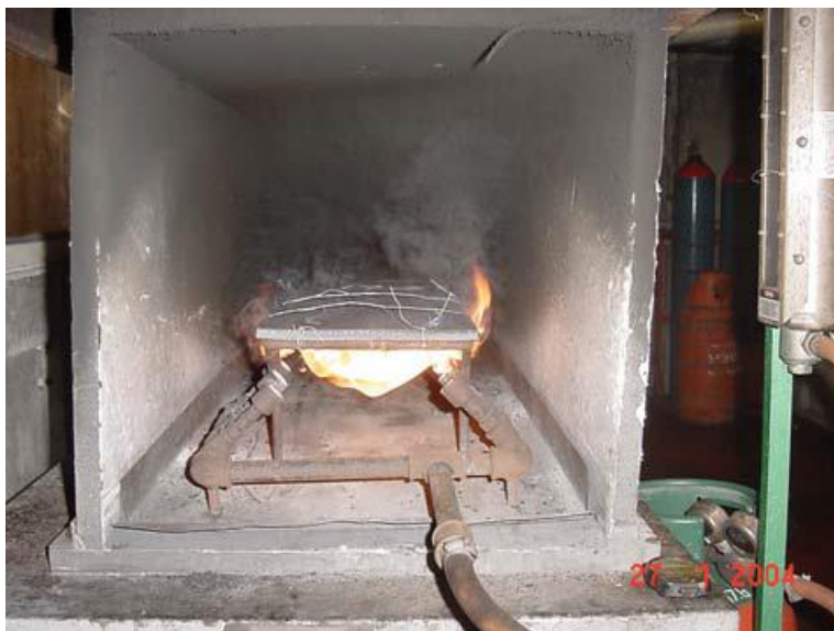
Figure 4. EN 12881-1. Method C. Test gallery.
