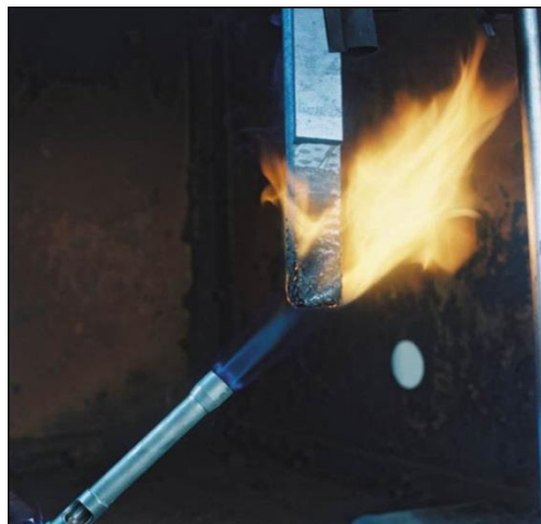
Figure 1. SANS/ISO 340 test burner flame at 1 000 °C 2 .
