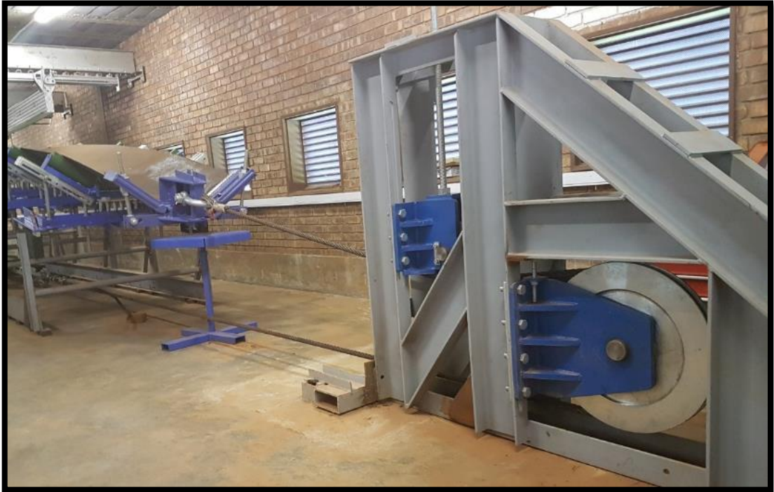
Figure 5. Image of the sheave structure and belt attachment.
