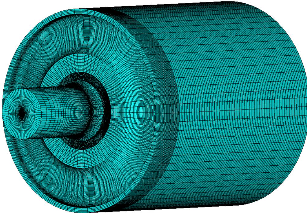
Figure 9. ANSYS 3D Element Plot of Pulley
