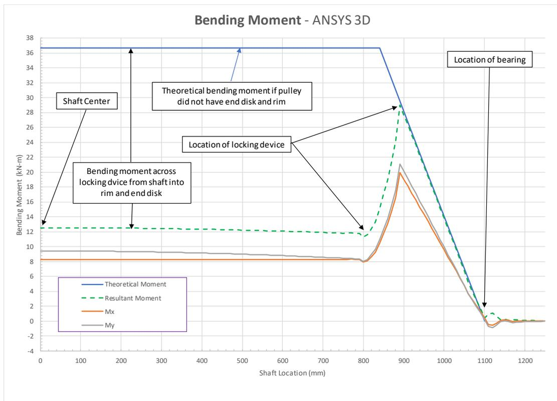
Figure 3. Bending moment calculation from finite element model
