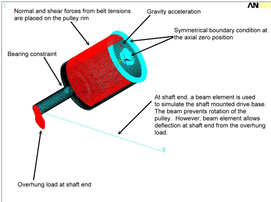
Figure 2. Boundary conditions of symmetrical drive pulley
