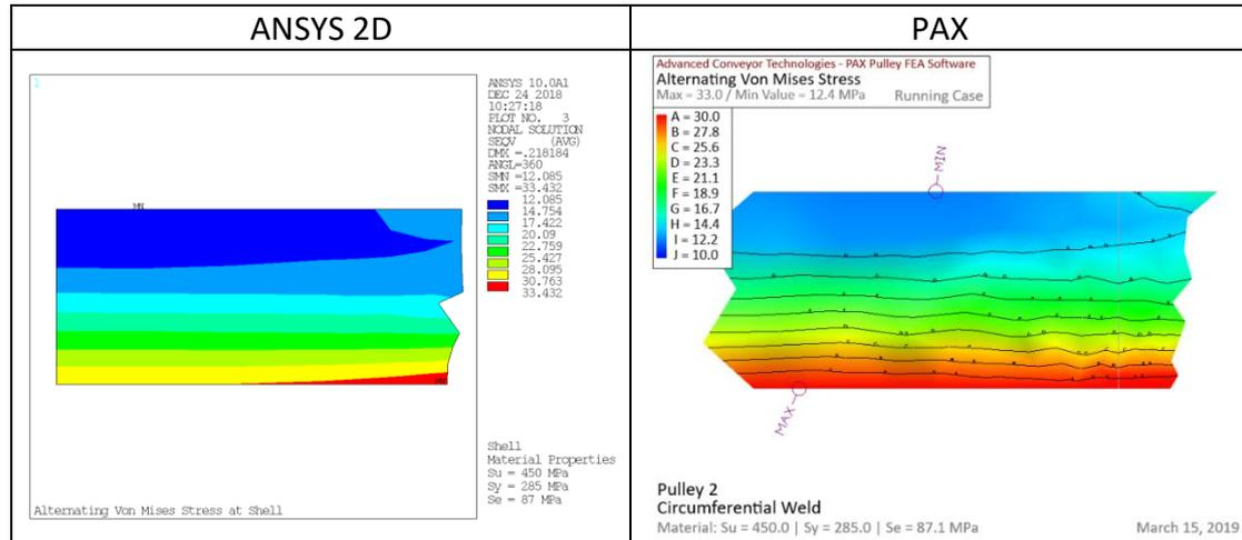
Figure 12. Alternating stress at inside edge at the weld location between rim and end disk
