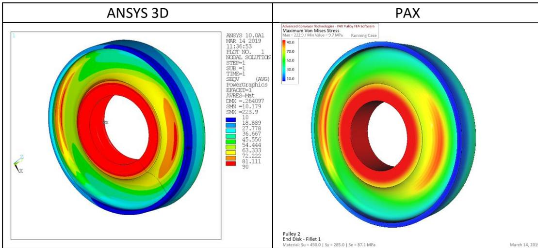
Figure 15. Von mises stress in end disk
