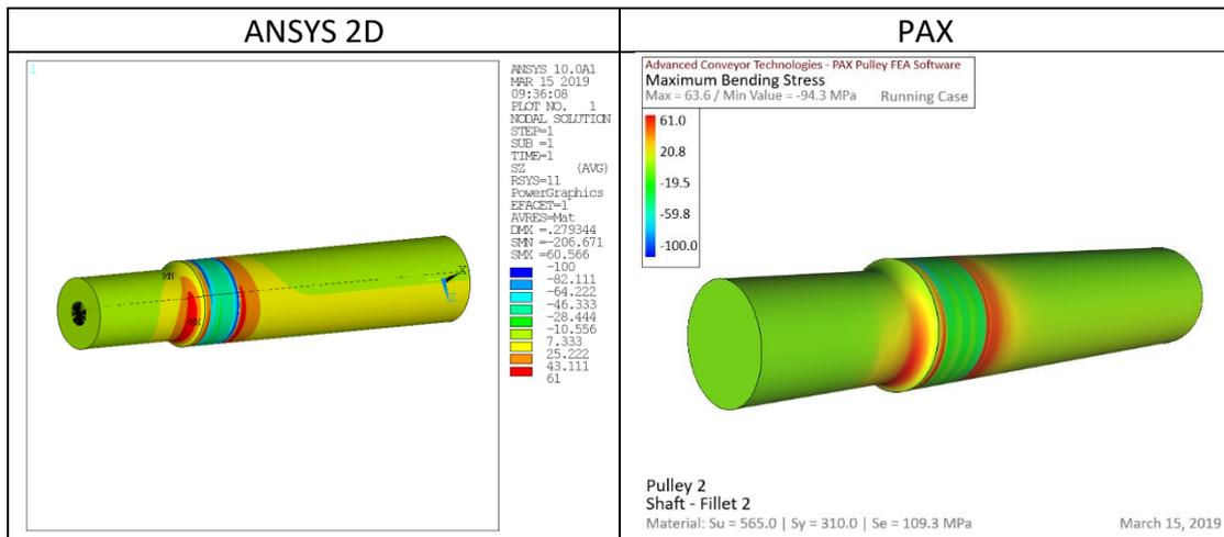
Figure 18. Axial (bending) stress in shaft
