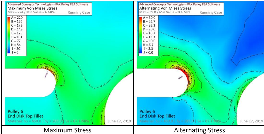
Figure 26. Alternating von mises stress in the weld (PAX)
