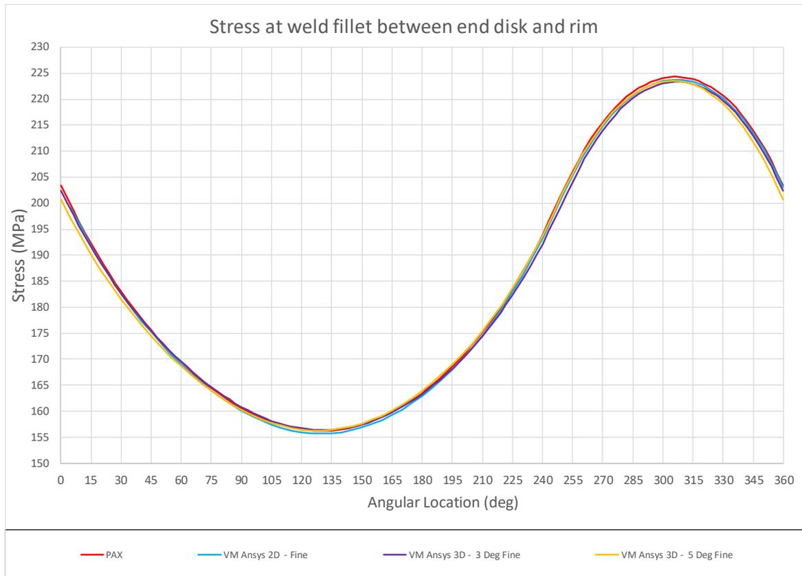
Figure 30. Von Mises stress at fillet weld between end disk and rim with refined 3D model
