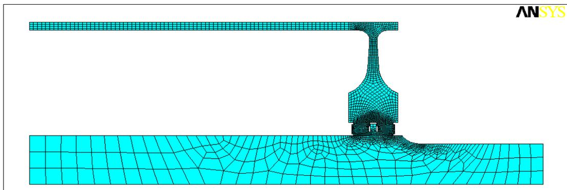
Figure 8. ANSYS 2D Element Plot of Pulley
