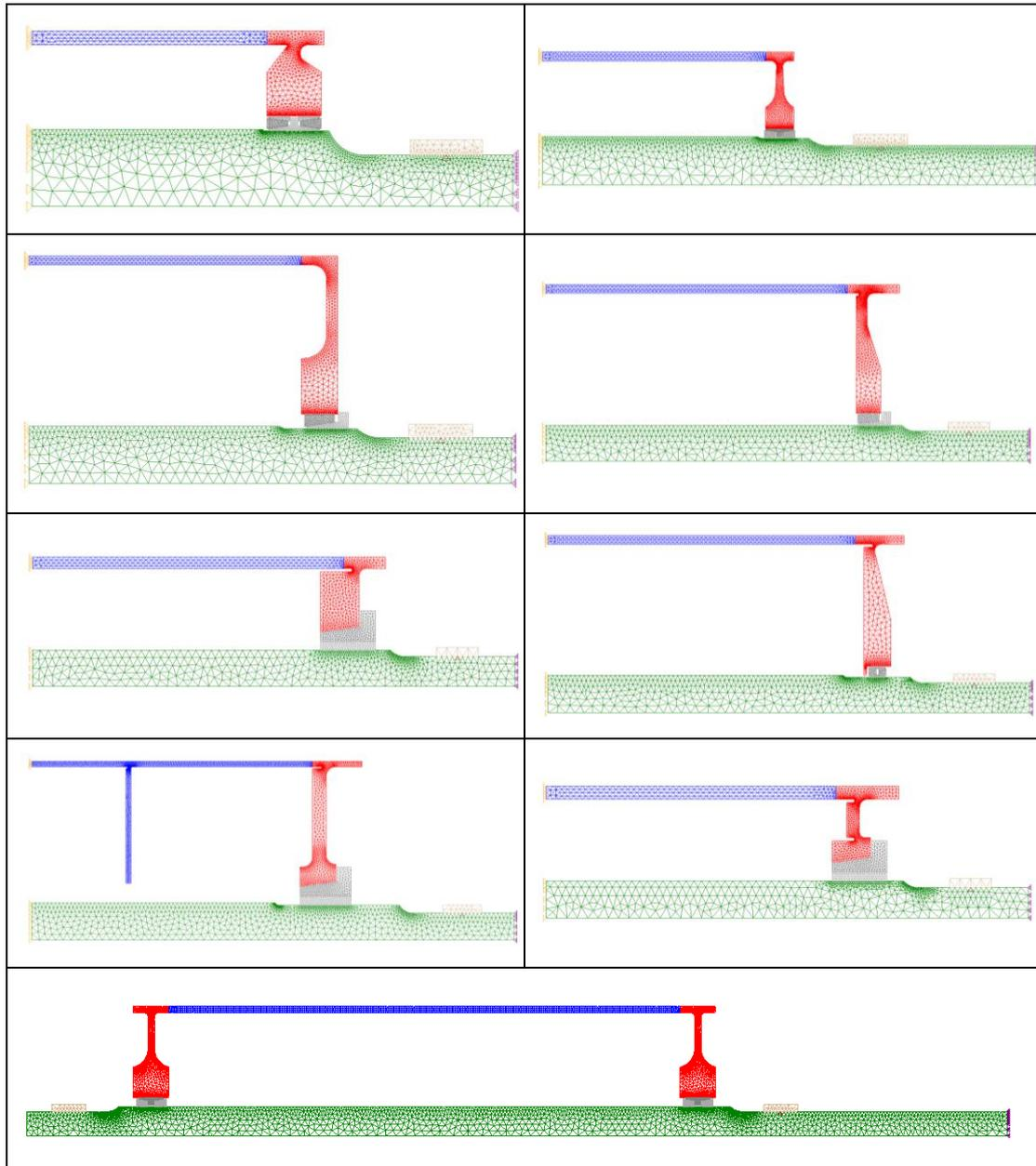
Figure 20. Various pulley geometries analysed using full 3D and 2D axis-symmetric elements
