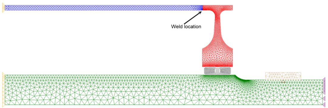
Figure 7. PAX Element Plot of Pulley
