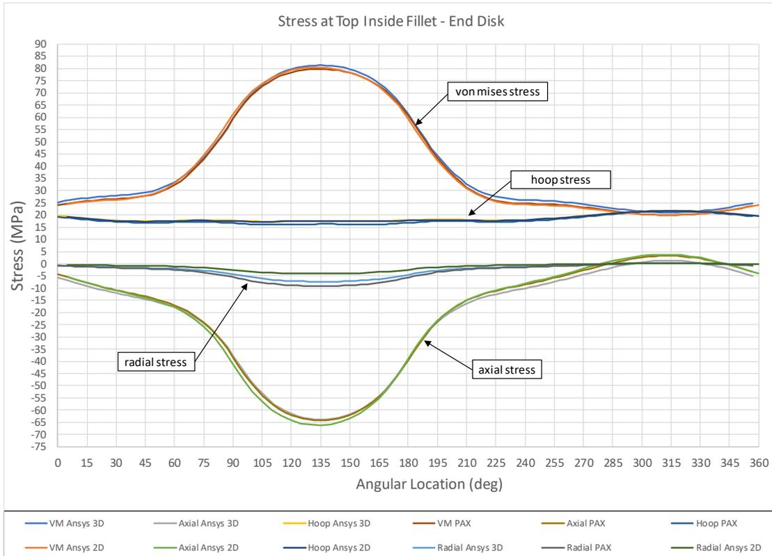
Figure 14. Stress at top inside fillet in the end disk
