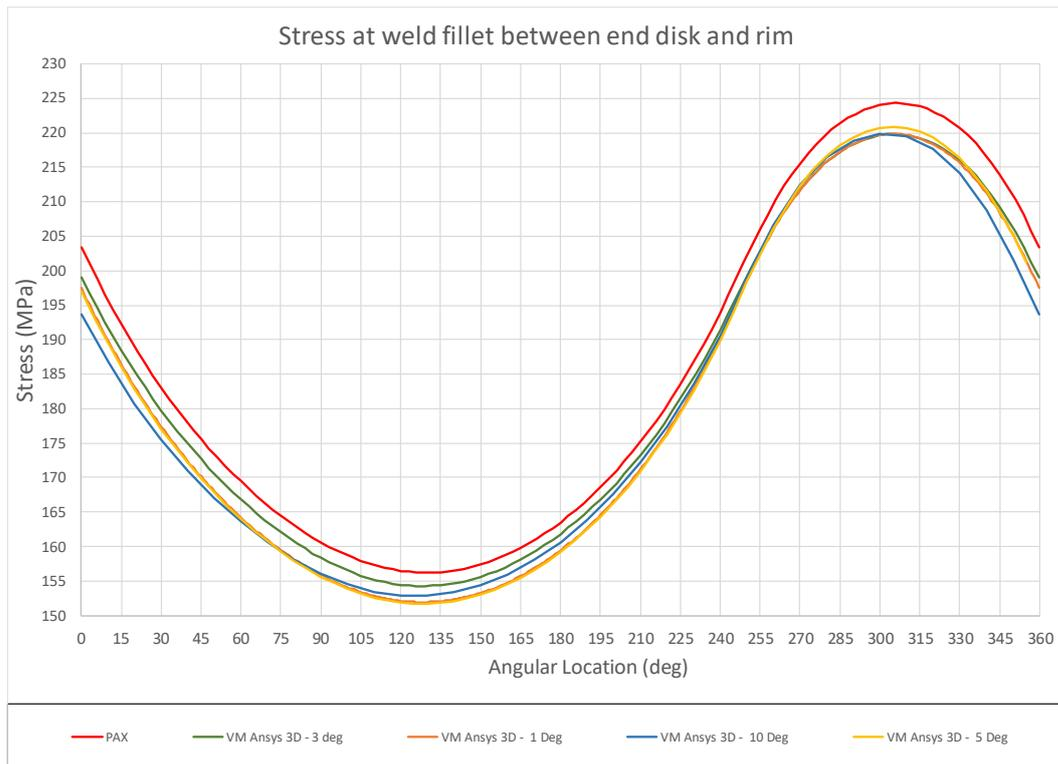
Figure 28. Von Mises stress at fillet weld between end disk and rim
