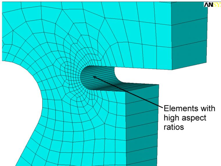
Figure 27. 3D elements at weld fillet (5 degree element rotation angle)
