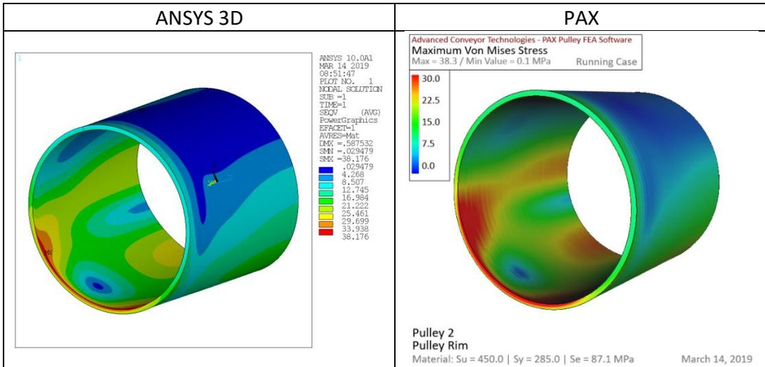
Figure 11. Stress at inside edge at the weld location between rim and end disk
