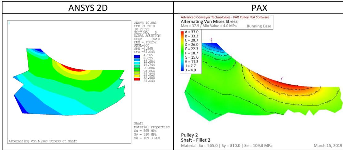
Figure 16. Alternating stress at bearing fillet in shaft
