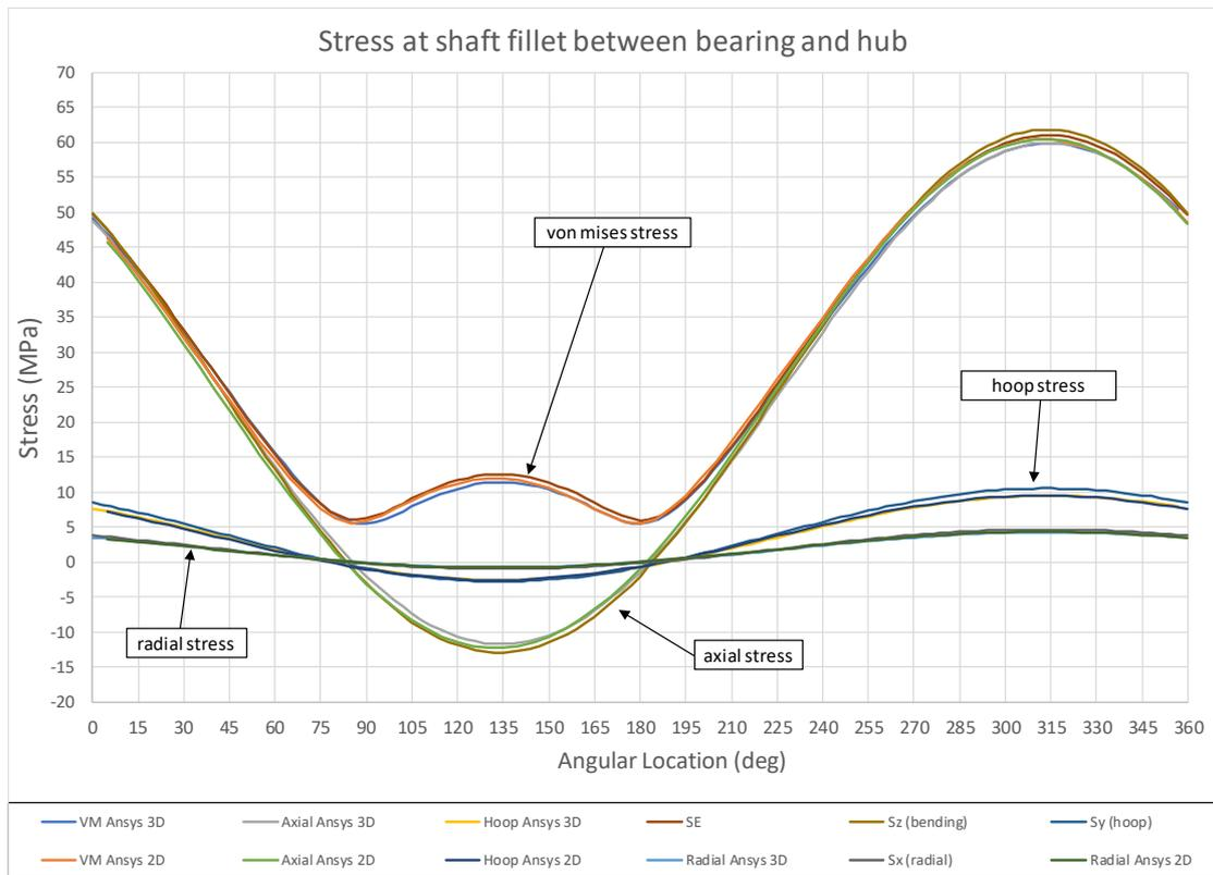
Figure 17. Stress at shaft fillet between bearing and hub
