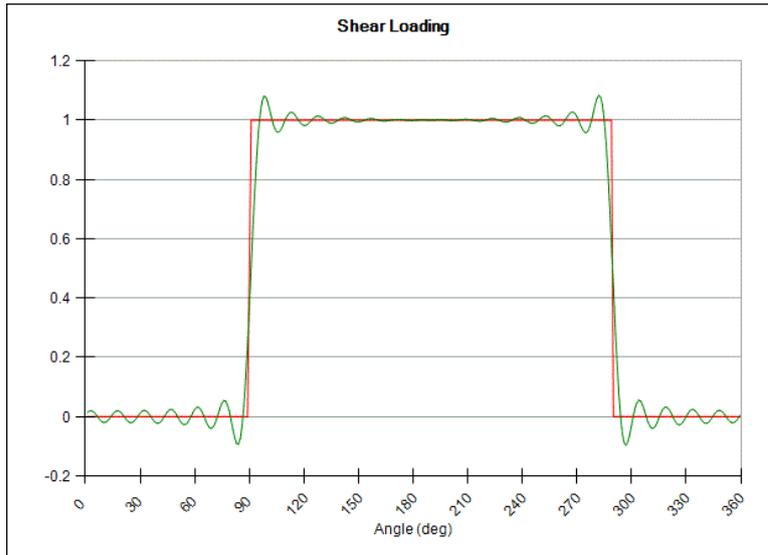
Figure 6. Shear Pressure Fourier Series (24 coefficients)
