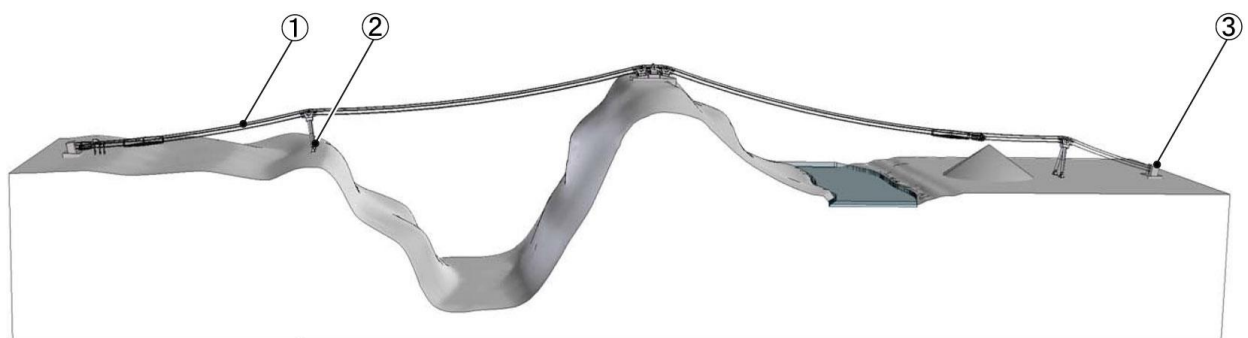
Figure 5: Typical RopeCon line structure; (1) Track ropes, (2) Tower and (3) Track Rope Anchor (Khodadadi, 2018).
