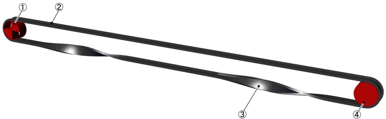
Figure 6: Typical RopeCon conveyor belt; (1) Drive pulley, (2) flat belt with corrugated side walls, (3) belt turning and (4) tail or return pulley (Khodadadi, 2018).
