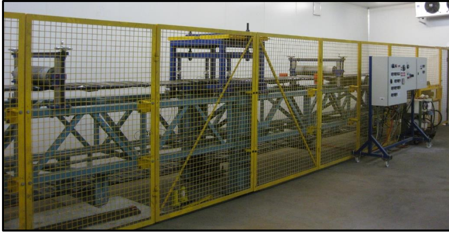
Figure 1 The University of Newcastle's indentation rolling resistance test machine inside its temperature controlled room [6].
