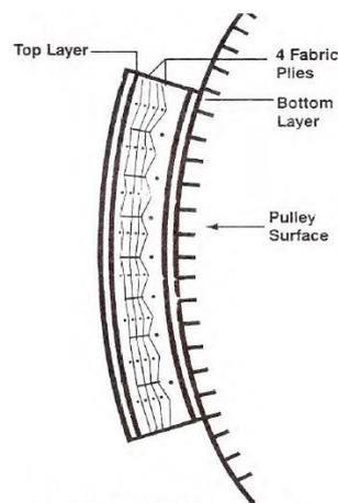
Figure 1: Ply Separation Failure due to Increased Stress around the Pulley (Dunlop Belting, n.d.)
