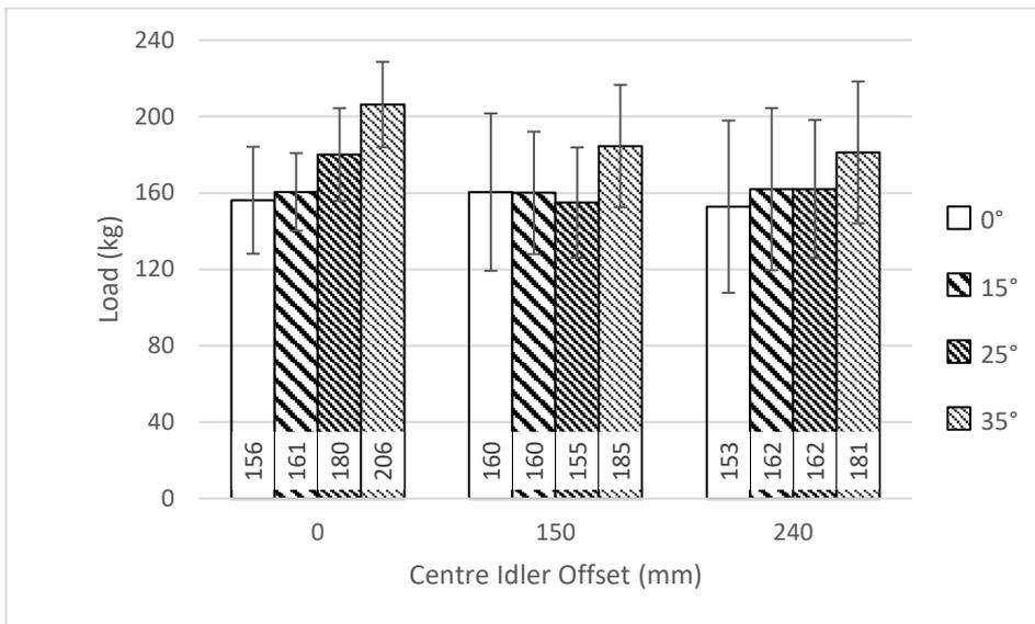
Figure 13: Average centre idler loads of all troughing angles and idler offset - pseudo-dynamic loading case
