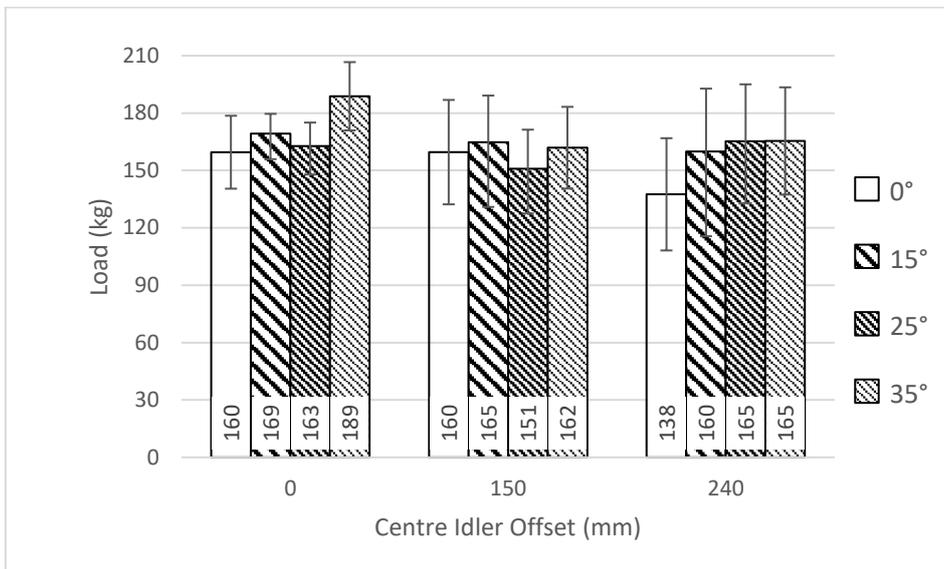
Figure 11: Average centre idler loads of all troughing angles and idler offset - static loading case
