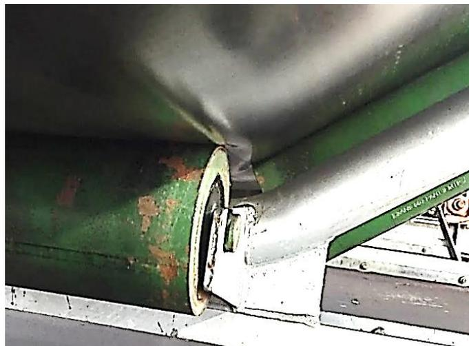
Figure 3: Belt friendly idler frame - creasing of the belt between the idlers (Kruse, 2019)
