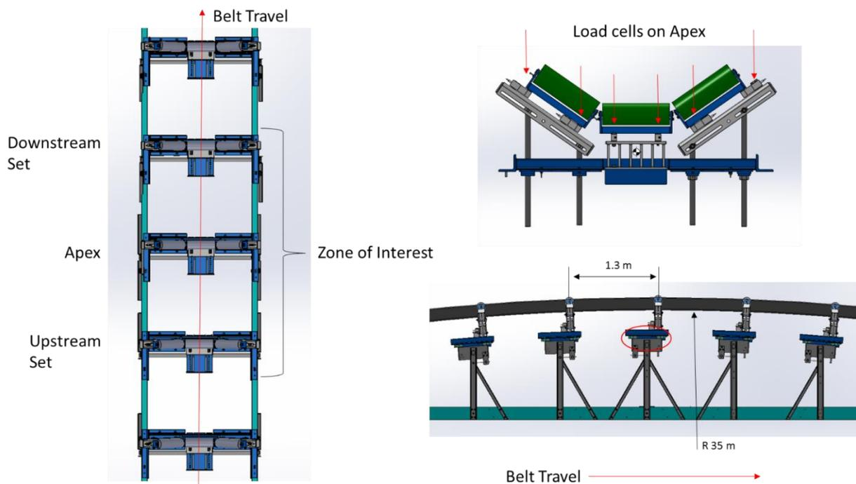
Figure 8: Load cells in the zone of Interest
