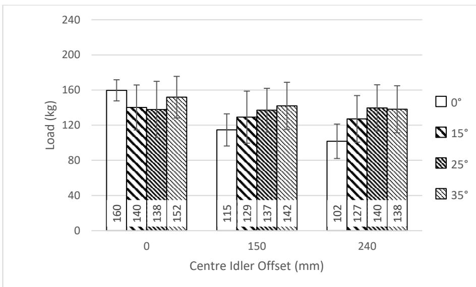
Figure 14: Average wing idler loads of all troughing angles and idler offset - pseudo-dynamic loading case
