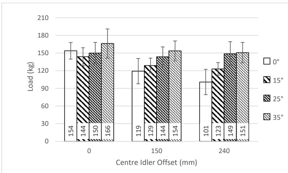
Figure 12: Average wing idler loads of all troughing angles and idler offsets - static loading Case
