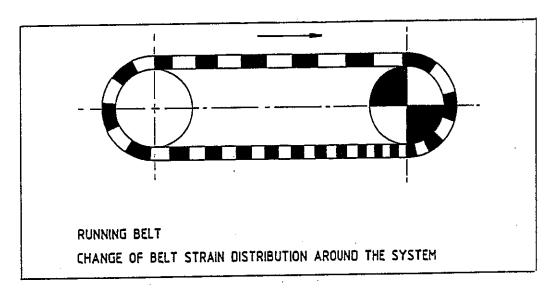
The function of the screw-type take-up is to pre-stretch the belt such, that the tension in the belt is equal to the calculated average tension required for the system.
