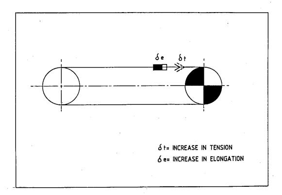
On energising the drive motor the torque at the drive pulley will increase the tension in the belt until this tension equals the total resistance of the system. At this point the belt will begin to move. To maintain belt movement will not require any further increase in tension.
