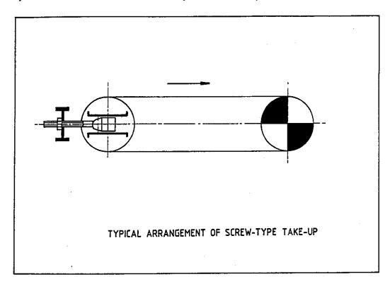
On longer conveyors perhaps the most common take-up system is the gravity take-up device. However, with the developments of long, high-capacity conveyor systems, even gravity take-ups have their limitations. This has led to the introduction of automatic power take-up systems.
