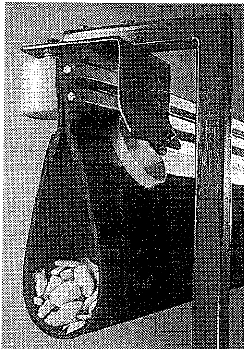
Figure 1 - Cross Section of the SICON belt.
