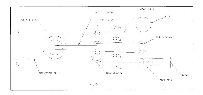
Mechanical tension sensing has a very limited range and is generally not considered an option particularly as the two set point method which is used with mechanical dynamometers causes hunting in the system. This will lead to winch motor burn outs with consequent down time and maintenance costs.
